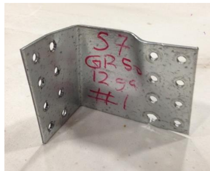
Figure 2.6: Test result of clip angle S7 #1
