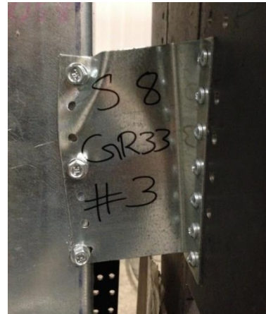
Figure 2.5: Test result of clip angle S8 #3
