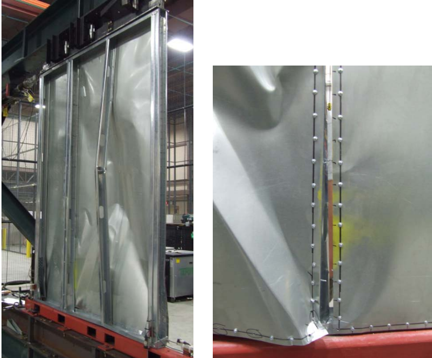
Figure 17 Failure mode of test 8x6x350-43x30-2-C1-A
