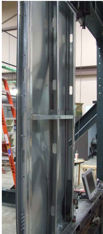
Figure 25 Failure mode of test 8×4×350-43×33-2-C1-C
