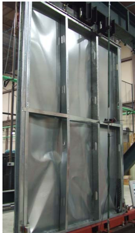
Figure 21 Failure mode of test 8×6×350-43×33-2-C1-C
