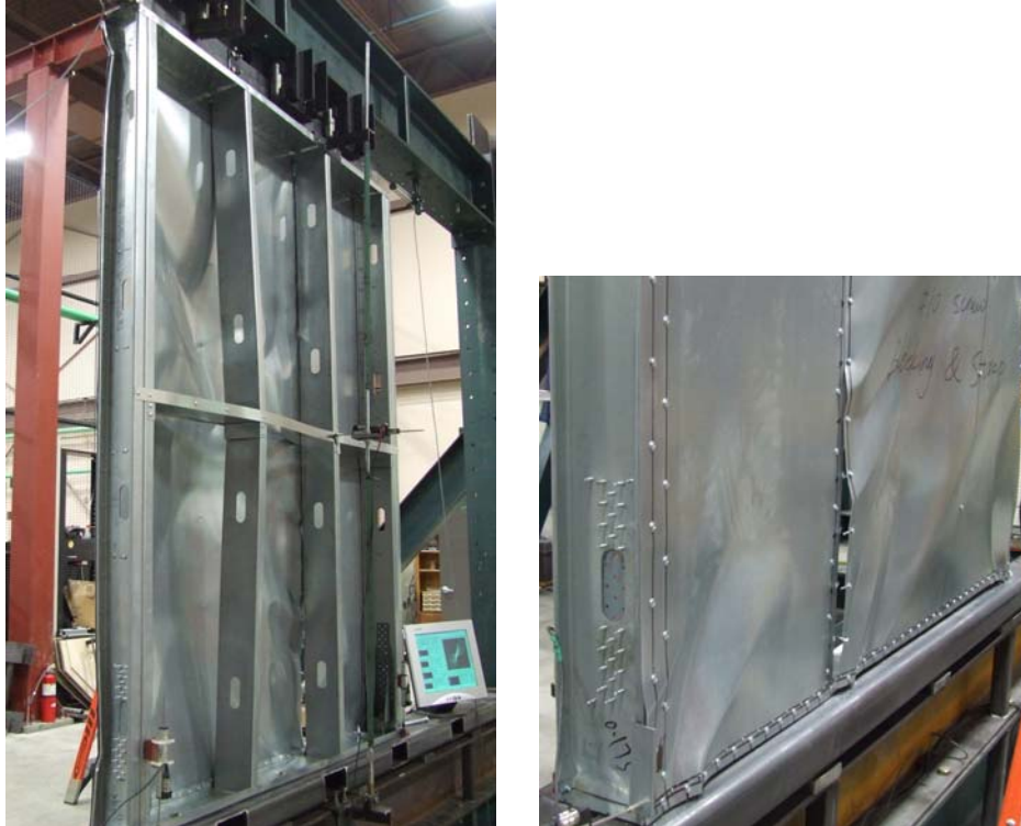
Figure 22 Failure mode of test 8x6x600-43x30-2-C1-C
