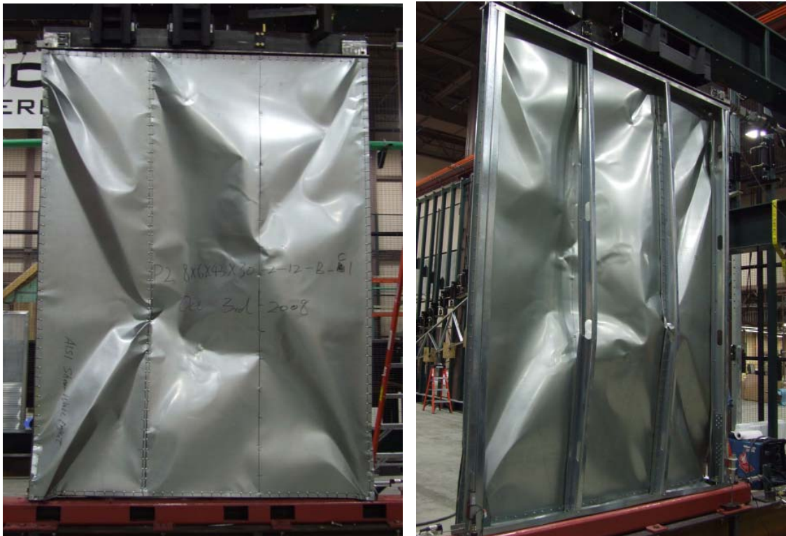
Figure 19 Failure mode of test 8x6x350-43x30-2-C1-B
