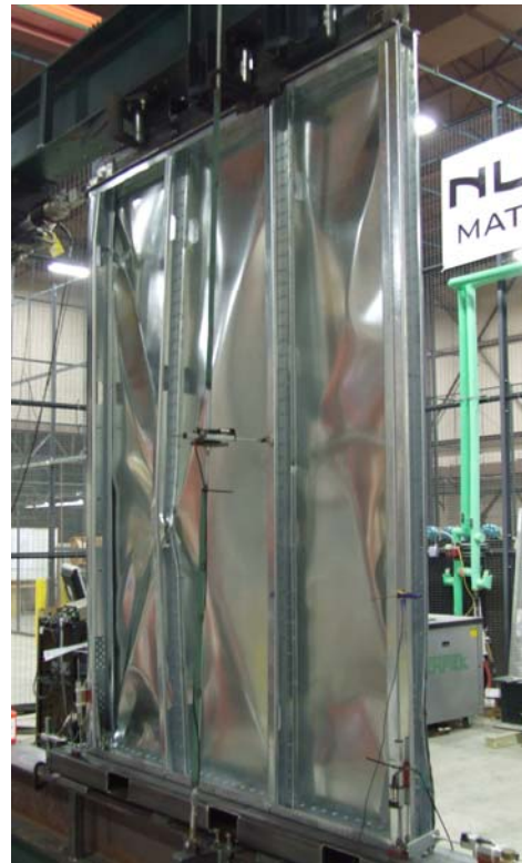
Figure 29 Failure mode of 8x6x350-43x27-2-C1-D
