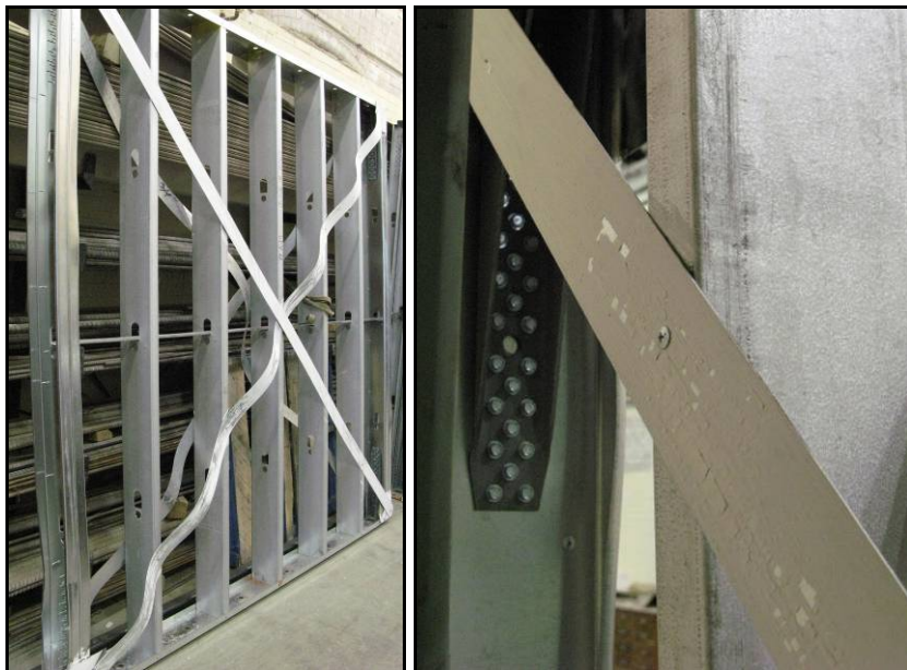
Figure 2.23: Medium walls showing brace yielding
