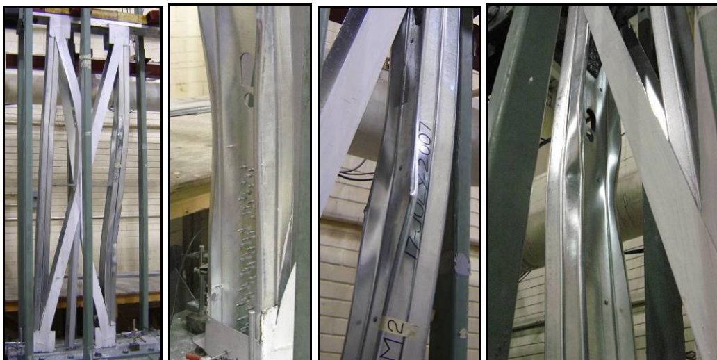
Figure 2.25: Chord stud failure in specimens 19B-M1 and 19B-M2
