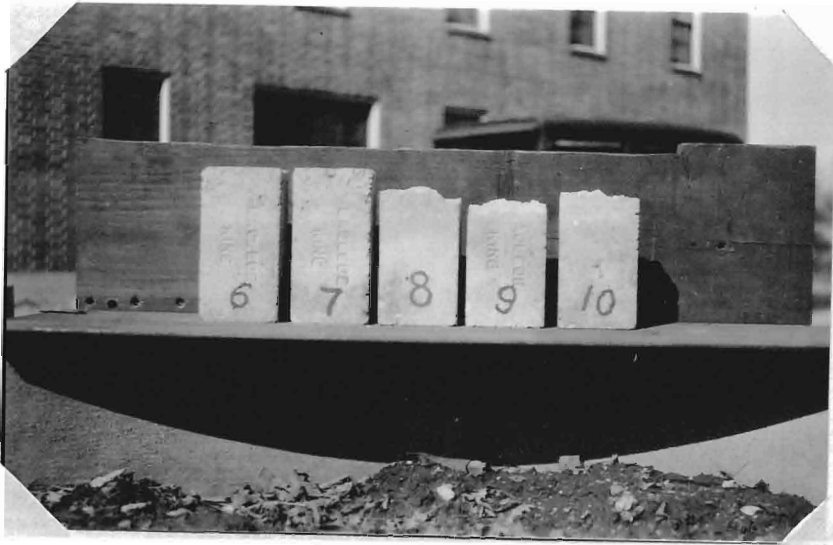
Figure 3 Laclede King Brick after subjection to the Federal Specifications Spall Test.
