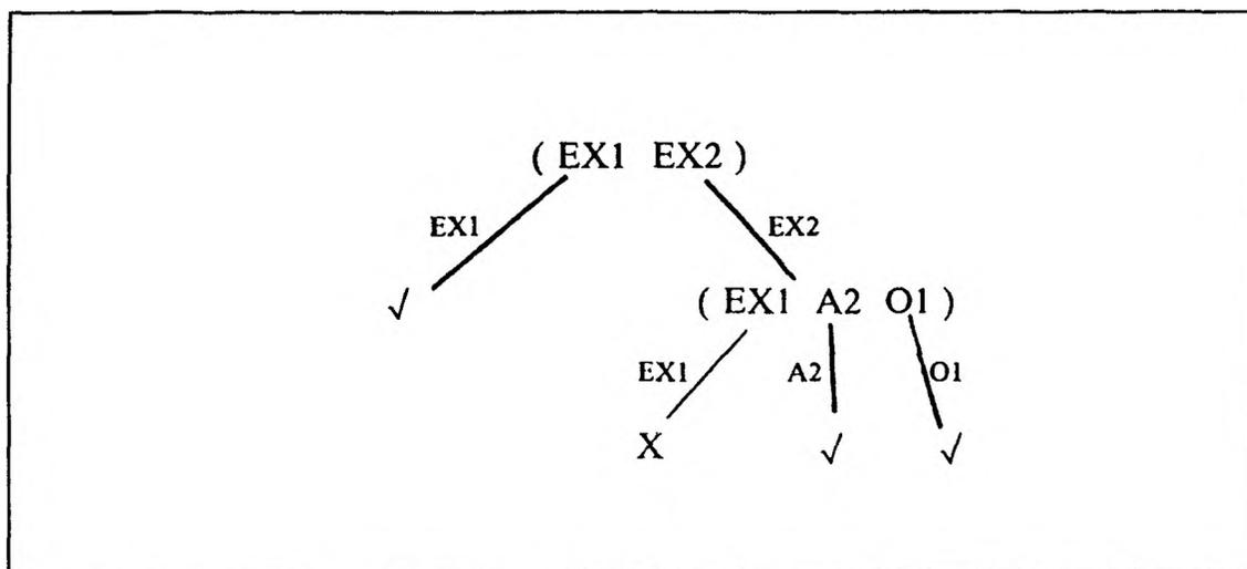
Figure 6. A hitting set tree for diagnosing the full adder
