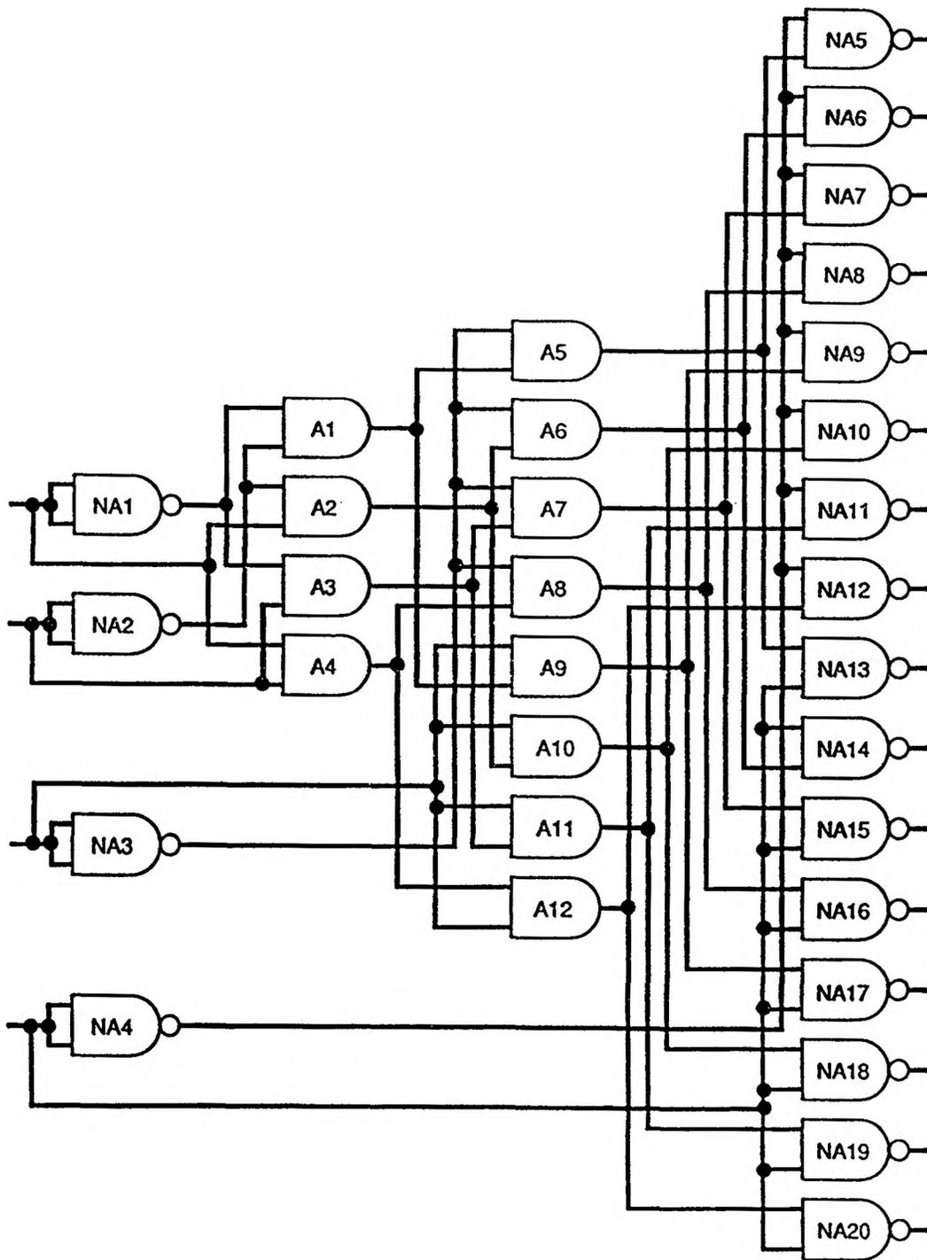
Figure 33. Diagram for a 4 to 16 line decoder
