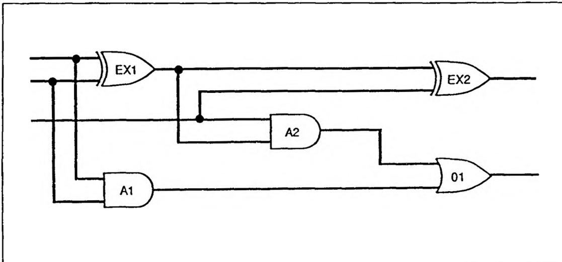
Figure 1. Diagram of a full adder
