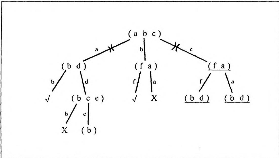
Figure 14. HS-tree with redundant edges marked
