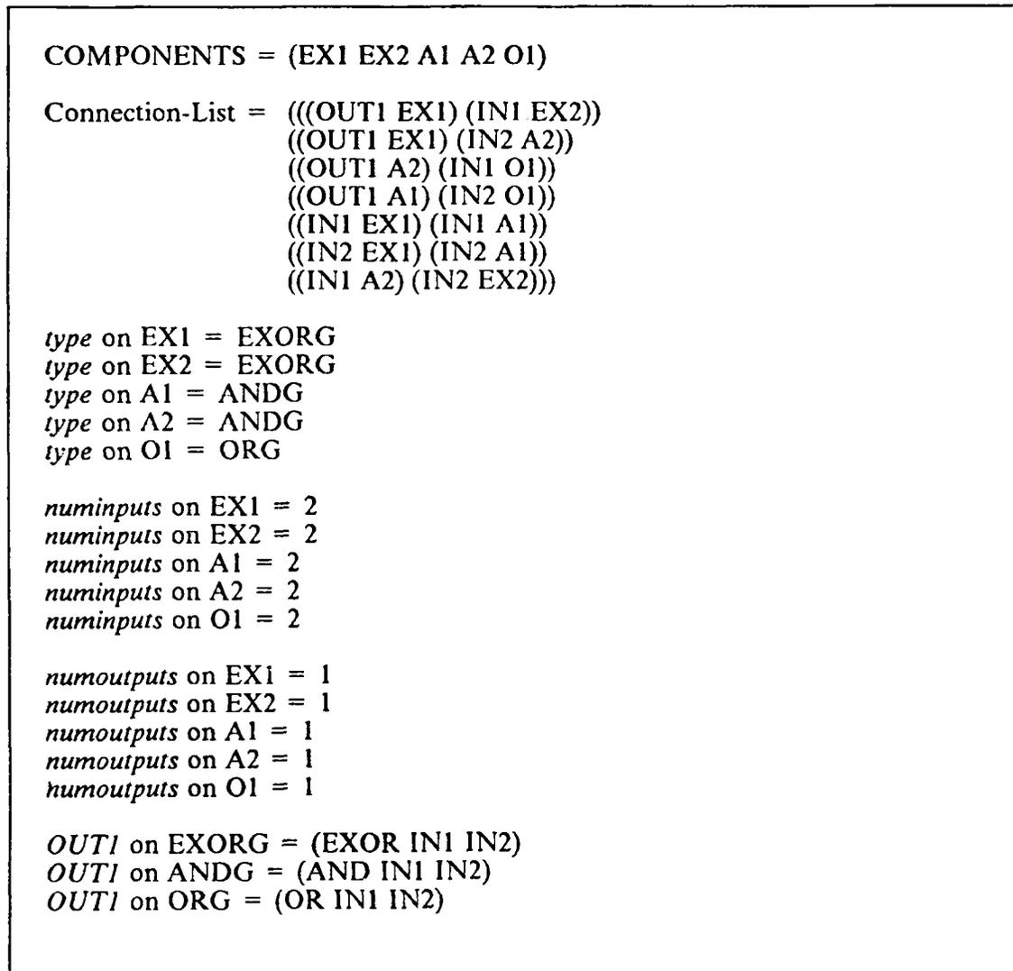
Figure 28. Representation of the full adder used in the implementation
