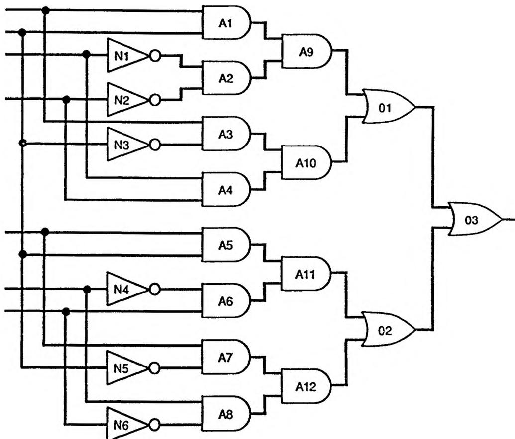
Figure 30. Diagram for an overflow detector
