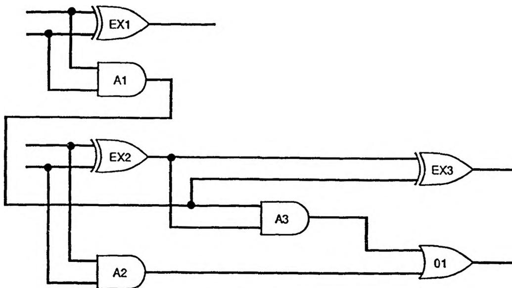
Figure 29. Diagram for the two bit adder
