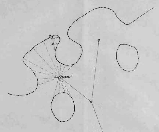
The preceeding of course applies only where a survey of the outline of the rough workings is desired. Where there is a property line to establish, or a drill hole to cut to, or two drifts to meet, the work must be carried right up with all the accuracy used in setting the permanent stations. Everything then must be kept in latitudes and departures, calculated as you proceed if need be. For instance, if we want to drift to a drill hole whose latitude and departure we know, from a surface survey
