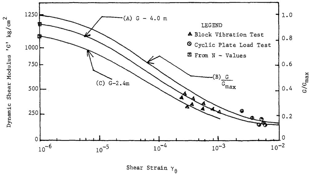
Fig. 4  $G$  vs  $\gamma_\theta$  and  $\frac{G}{G_{max}}$  vs  $\gamma_\theta$
