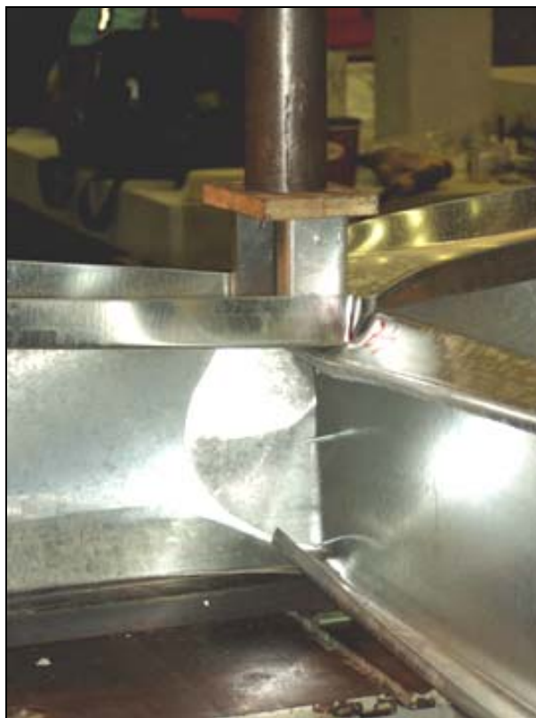
Figure 5.2: Photograph of Excessive Deformation
