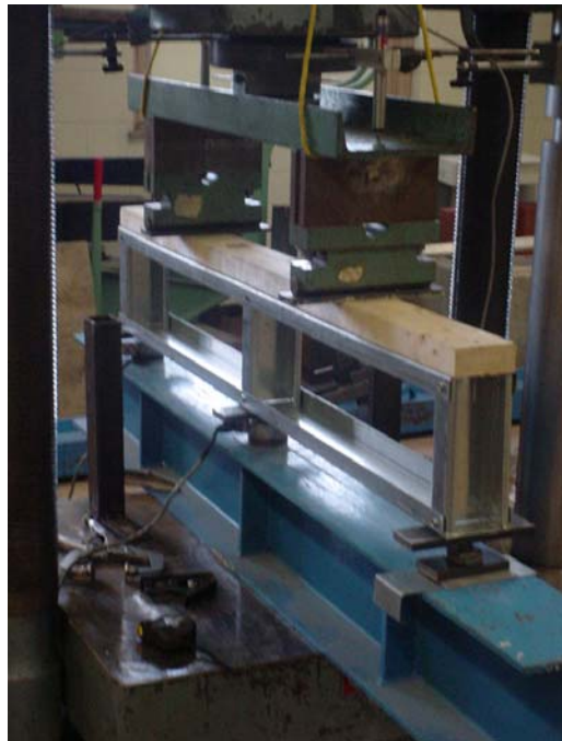
Figure 3.2 – Typical Test Setup of 24 Inch Specimen
