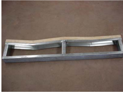
Figure 4.5 – Failed Specimen, 1A24-16
