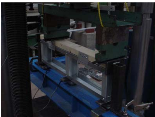
Figure 4.3 –Specimen 2A16-18 with shear plates
