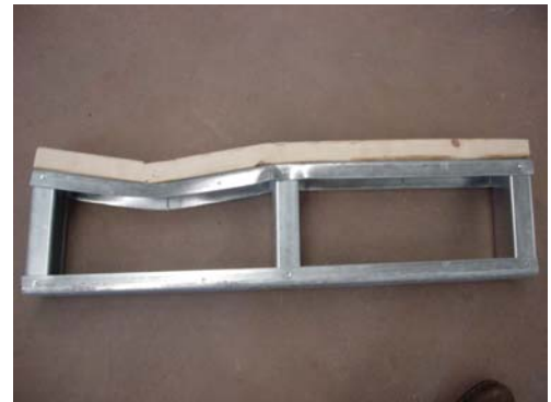
Figure 4.2 – Flexural failure of Specimen 1A16-18
