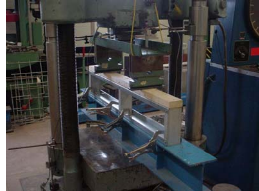
Figure 4.6 – Clamped Specimen, 3A24-18
