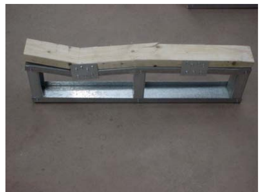
Figure 4.4 –Note wood/track separation
