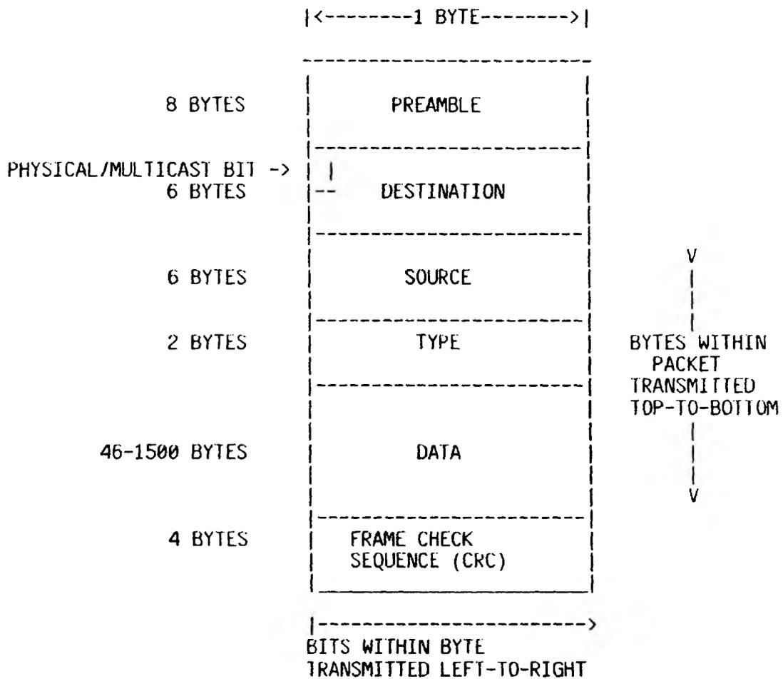
FIGURE 6 - ETHERNET PACKET FORMAT
