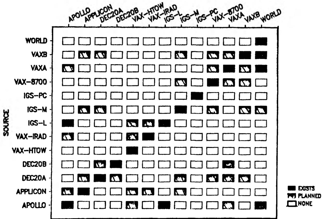
FIGURE 23 - EMERSON ELECTRIC FILE TRANSFER CAPABILITIES
