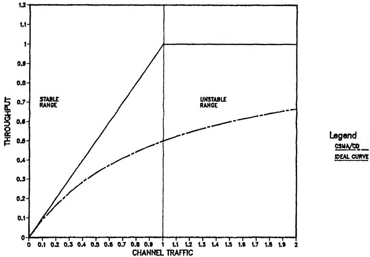
FIGURE 12 - SLOTTED NON-PERSISTENT CSMA/CD THROUGHPUT CURVE
