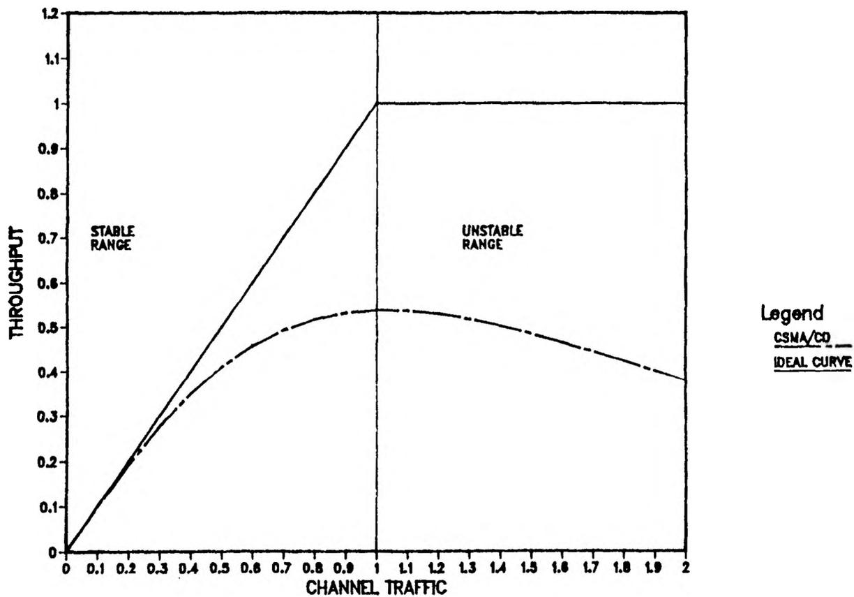
FIGURE 14 - SLOTTED 1-PERSISTENT CSMA/CD THROUGHPUT CURVE
