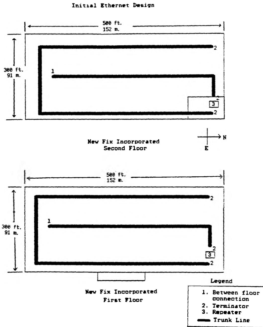
FIGURE 19 - DESIGN STUDY (NEW FIX INCORPORATED) FLOOR PLAN
