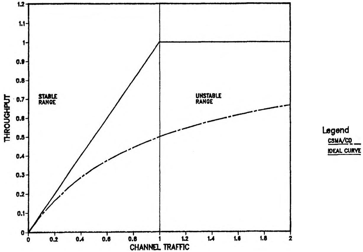
FIGURE 11 - NON-PERSISTENT CSMA/CD THROUGHPUT CURVE
