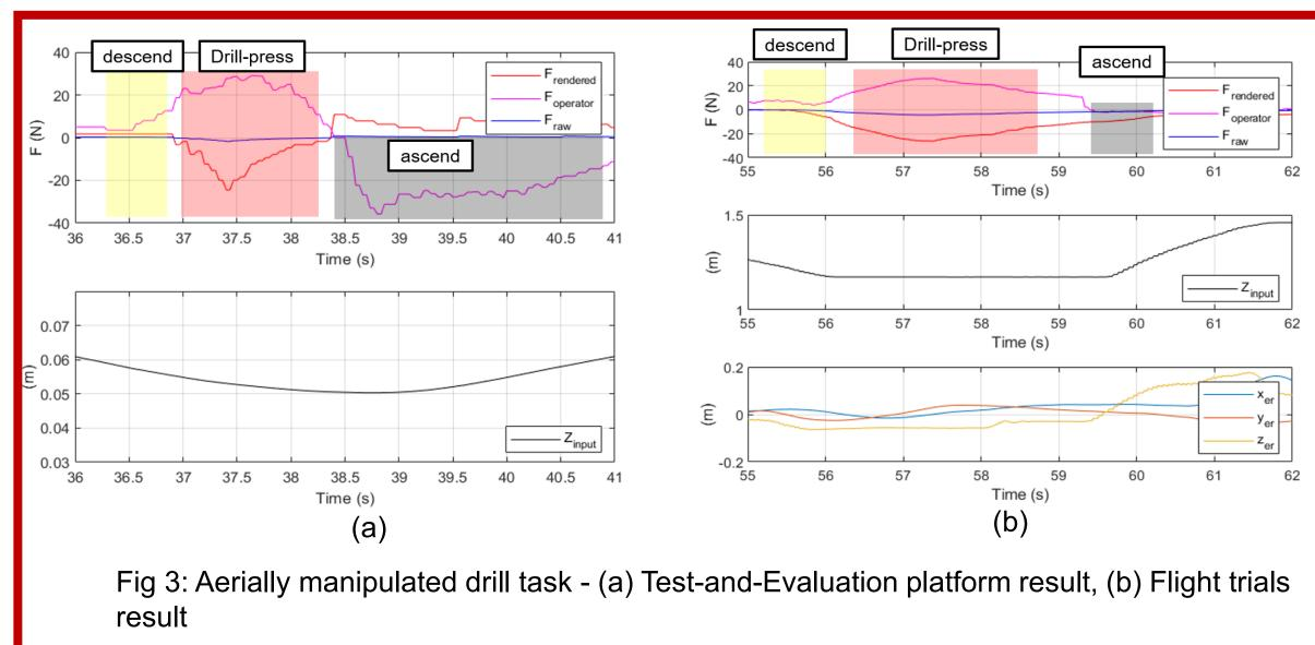
T&E and V&V results in Figure 3 successfully captured drillworkpiece contact forces. With these forces, the user was able to remotely drill through a variety of materials (e.g. wood and acrylic), of various thicknesses, and rates.
