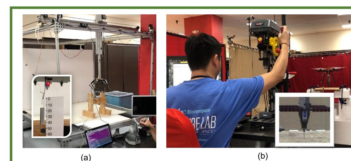
Fig 1: (a) shows Testing-and-Evaluation platform for haptic-based aerial manipulation, and (b) describes a proof-of-concept for human collaborative haptic-based aerial manipulation to perform surface work (Drilling)
