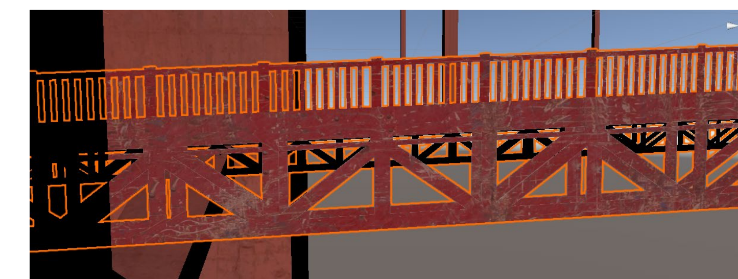
Software tools have been developed to map the truss structure of an existing bridge like the iconic Golden Gate bridge to the graph representation used by our optimizer for routing
