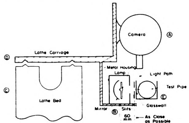
Figure 2. Photo-Optical System
