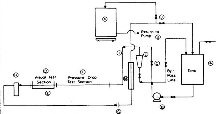
Figure 1. Schematic Diagram of Flow System
