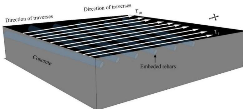
Figure 5: Illustration of GPR and PSPA traverses direction with respect to embedded concrete reinforcements
