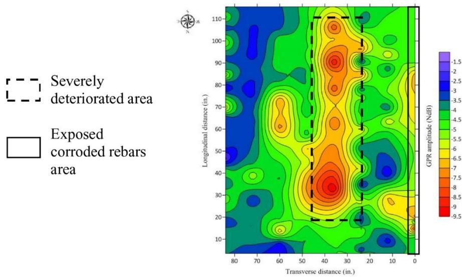
Figure 10: Amplitude variations map using 1.6 GHz (bottom section)
