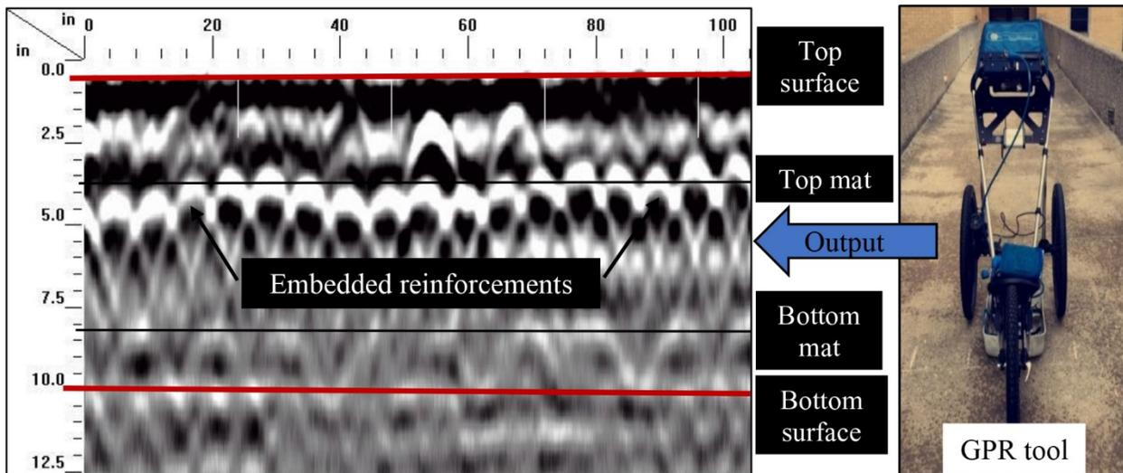
Figure 7: An example of processed GPR output showing embedded concrete reinforcements
