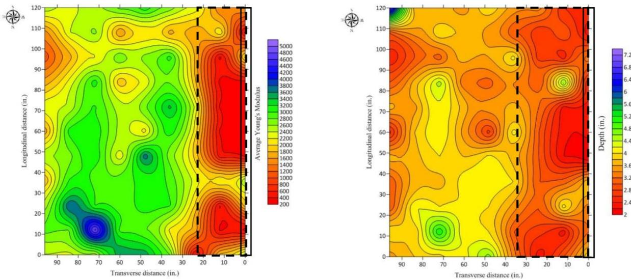
Figure 12: USW (left) and IE (right) variation maps (bottom section)
