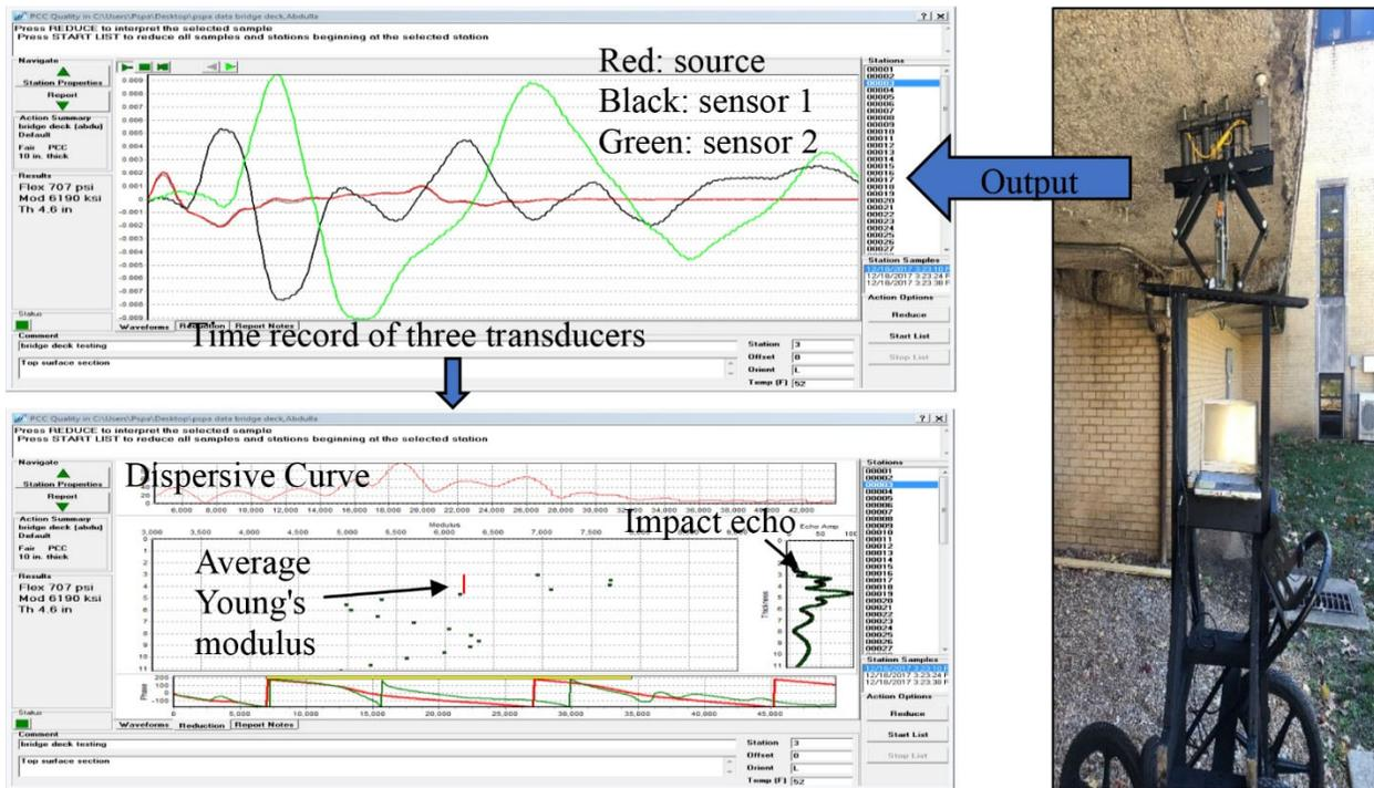
Figure 8: An example of processed PSPA output showing USW and IE results
