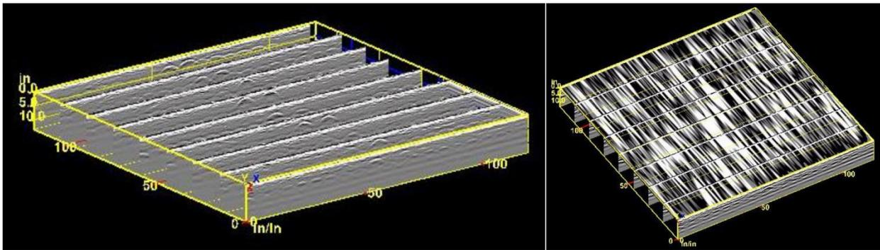
Figure 6: Illustration of GPR parallel profiles (left) and possible detected reinforcements (right) of top surface section using 2.5 GHz frequency antenna
