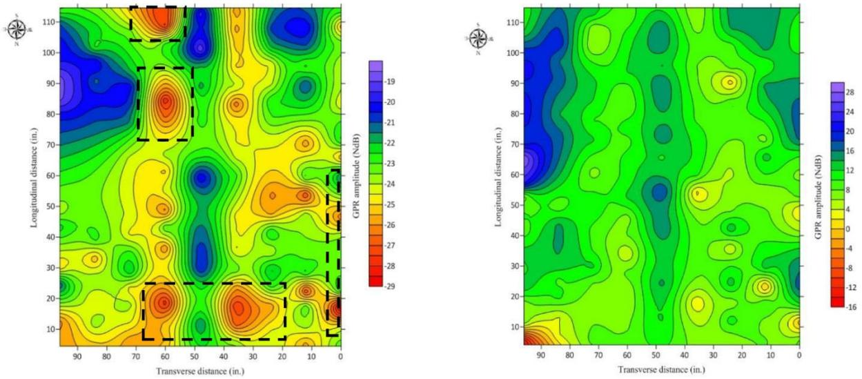
Figure 9: Amplitude variations map using 1.6 GHz (left) and 2.5 GHz (right) frequency (top section)
