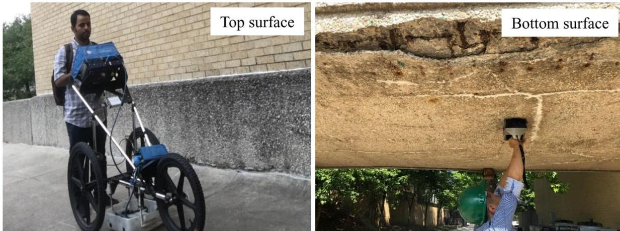
Figure 3: GPR data acquisition
