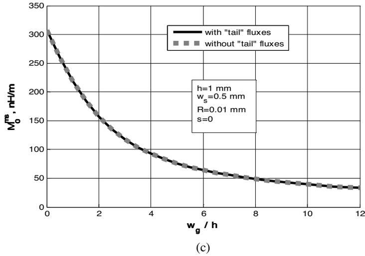
**Figure 5.** Mutual external inductance associated with the fringing magnetic fields wrapping the ground plane for a centered microstrip geometry: (a) at larger ratios  $w_g/h$ ; (b) at smaller ratios  $w_g/h$ ; (c) with and without the “tail current” flux accounted for.
