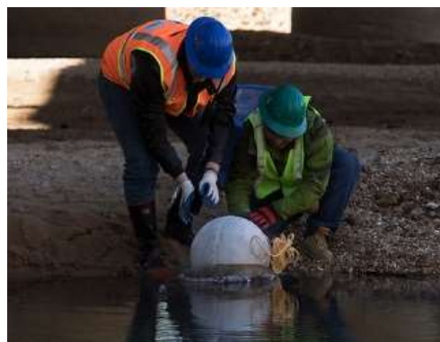
Figure 2 Fabricated smart rock and its deployment
