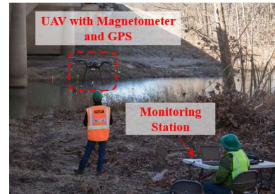
Figure 7 Smart rock positioning through UAV
