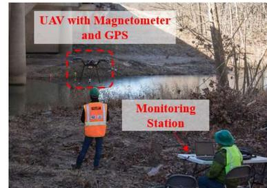
Figure 7 Smart rock positioning through UAV
