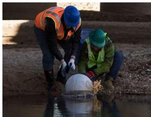
Figure 2 Fabricated smart rock and its deployment
