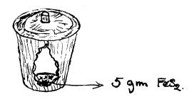
They were next placed in the muffle of an ordinary assay furnace and heated for one hour at temperatures varying from 100° to 900° C., the temperatures used being respectively 100°, 300°, 600°, 700°, 800°, and 900° C. After the roast was completed the crucible was placed in a bell jar of nitrogen to cool.
