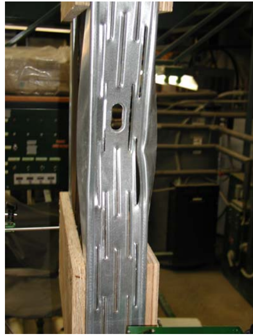
Slit-Web Stud Axial Test Setup and Failure Mode
