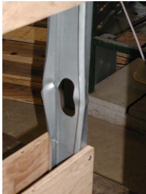
Solid Web Stud Failure Mode in Axial Tests
