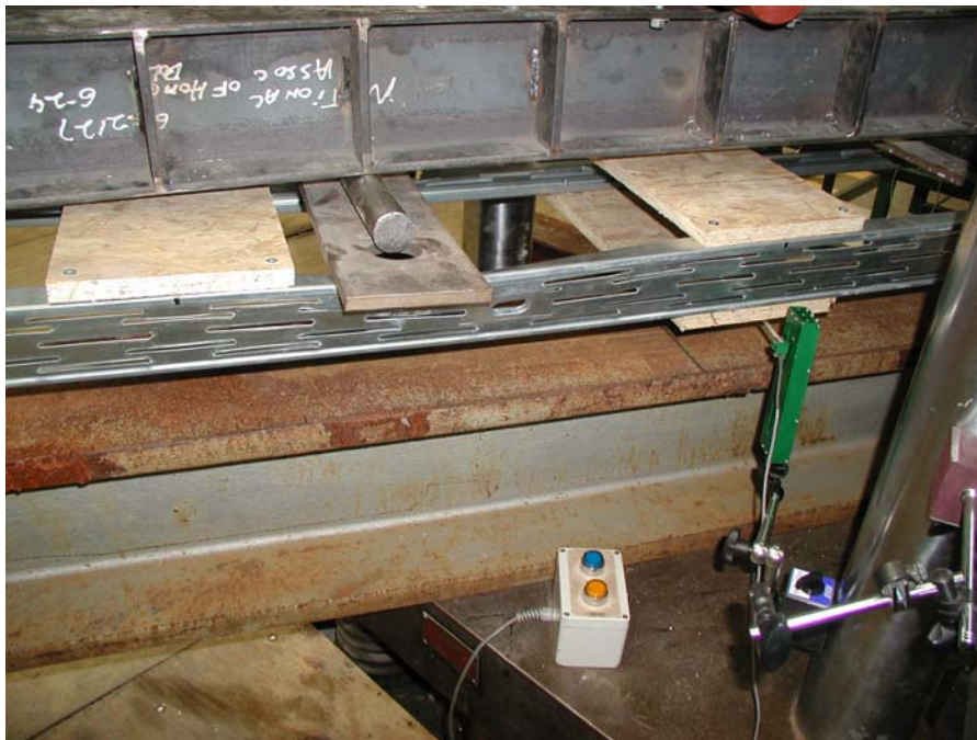
Failure of Slit-Web Stud in Bending Test
