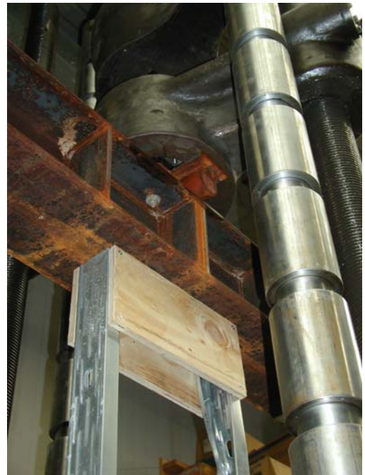
Slit-Web Stud Failure Mode in Axial Tests
