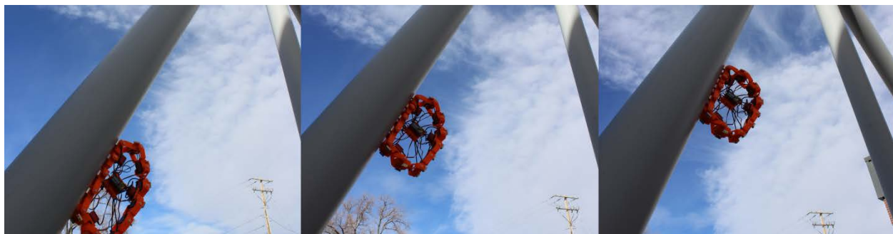
Fig 14. Climbing tests on a steel bridge at UNR's campus: https://www.youtube.com/watch?v=VoE4W5r_no&feature=youtu.be
