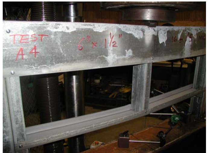
Figure 5 – Failure of Single L-Headers Tested Assemblies
