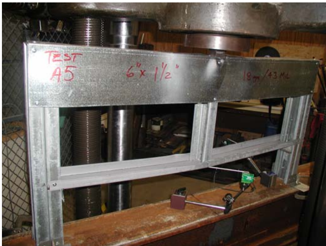
Figure 5 – Failure of Single L-Headers Tested Assemblies
