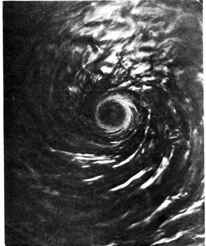
Fig. 7 Photograph of the unstable boundary layer beneath a concentrated vortex. Note spiral waves of instability and the central, non-rotating region.
