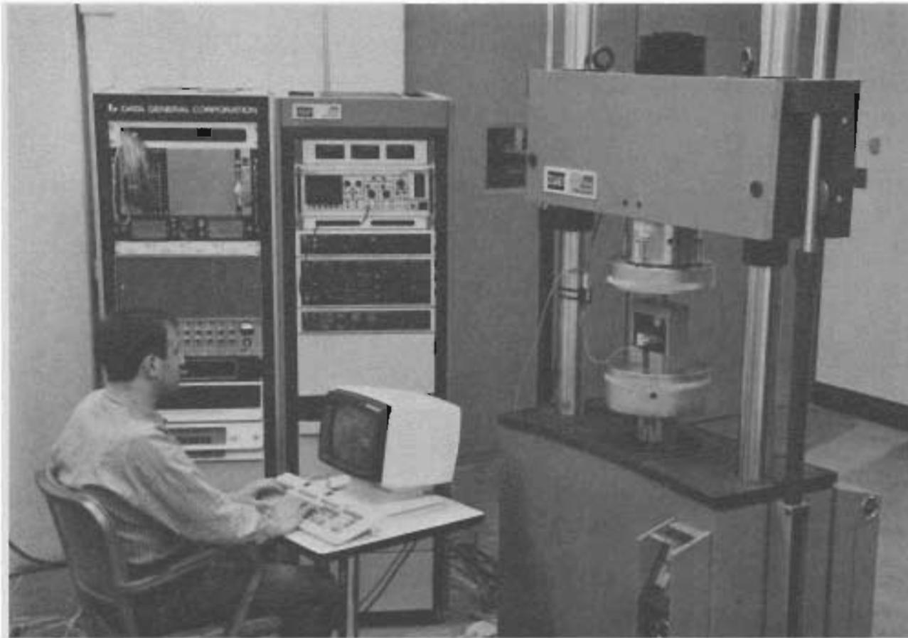
Fig. 3.3 MTS Load Frame, MTS Controller, CAMAC Data Acquisition System, and Data General Graphic Display Terminal Used for Compression Tests
