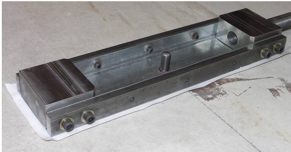
Figure 4: Close-up View of Test Fixture (Prior to Installation of Washer and Nut)
