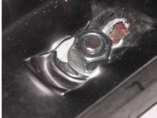
Figure 6: Monotonic Test with Standard Cut Washer
