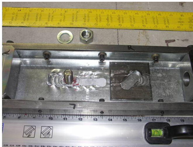
Figure 5: Monotonic Test with Plate Washer
