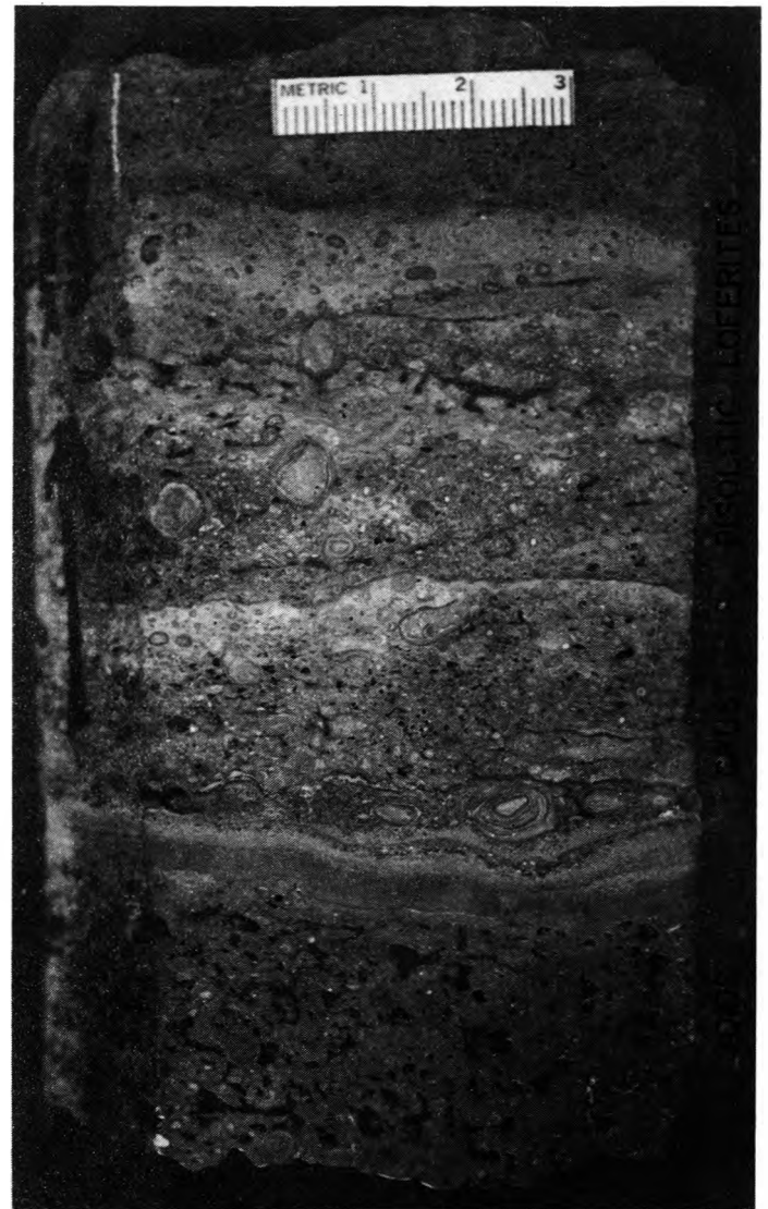
b. Loferite shrinkage or desiccation voids overlain by subaerial laminated crust, in turn overlain by pisolitic loferites. Texota #1 Weber at 4600 feet. Scale on photo is 3 centimeters long.
