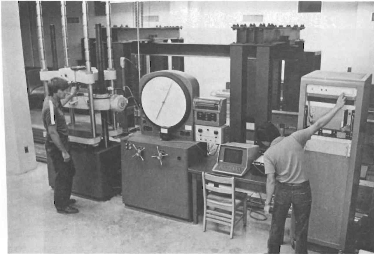
Fig. 3.5 Tinius Olsen Universal Testing Machine Used for Tension Tests 48
