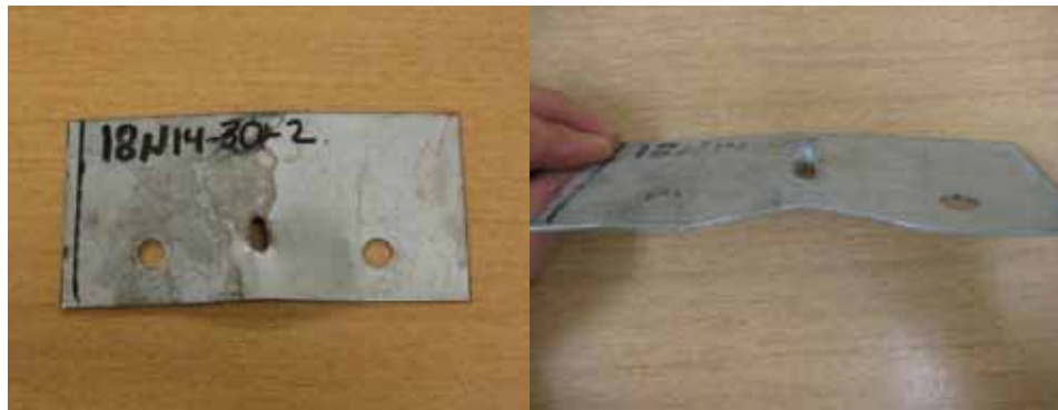
Figure 3.14 Typical Normal-Ductility Flat Sheet after Testing
