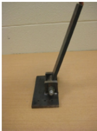
Figure 3.7 Lower Fixture: Rotating Arm
