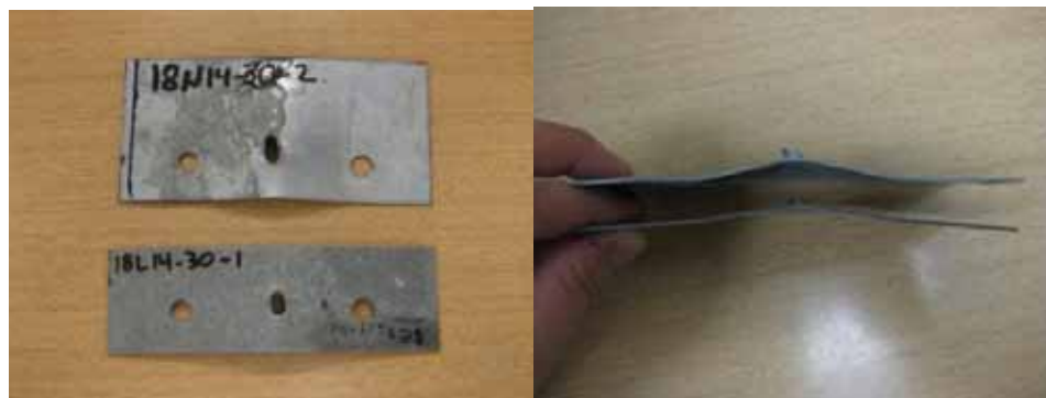
Figure 3.15 Comparison of Normal- and Low-Ductility Flat Sheets
