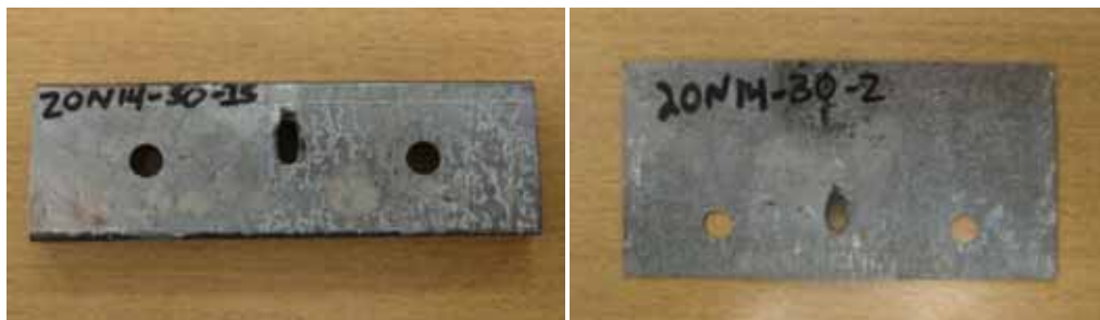
Figure 3.11 Comparison of Stiffened versus Un-stiffened Failure Modes
