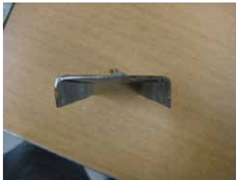
Figure 3.10 Flat Sheet with Edge Stiffeners
