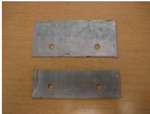
Figure 3.5 Normal- and Low-Ductility Flat Sheets
