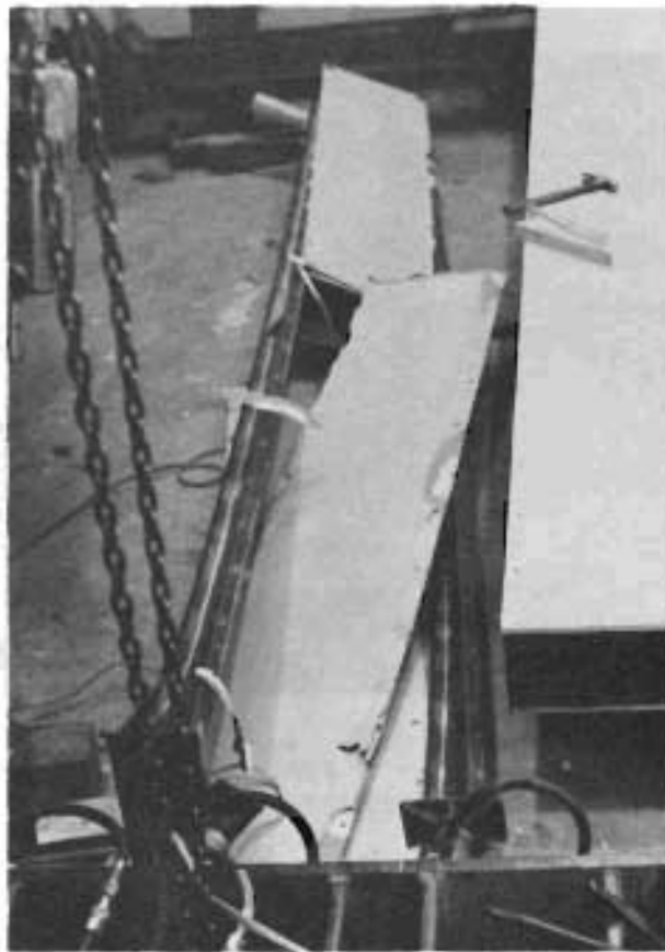
Photo 1 View of Test 1 - The specimen jumped out of the test fixture
