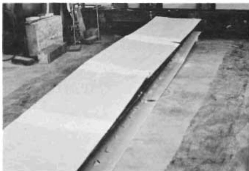
Photo 10 View of Test 5 - This test specimen had the largest initial sweep
