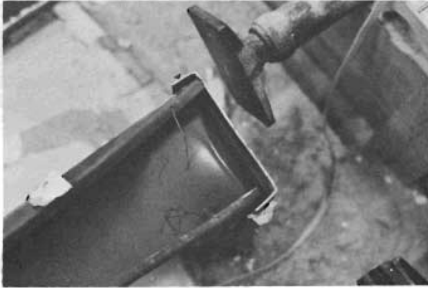
Photo 3 End Channels in Test 1 - The flanges opened up when the studs press against the round corners
