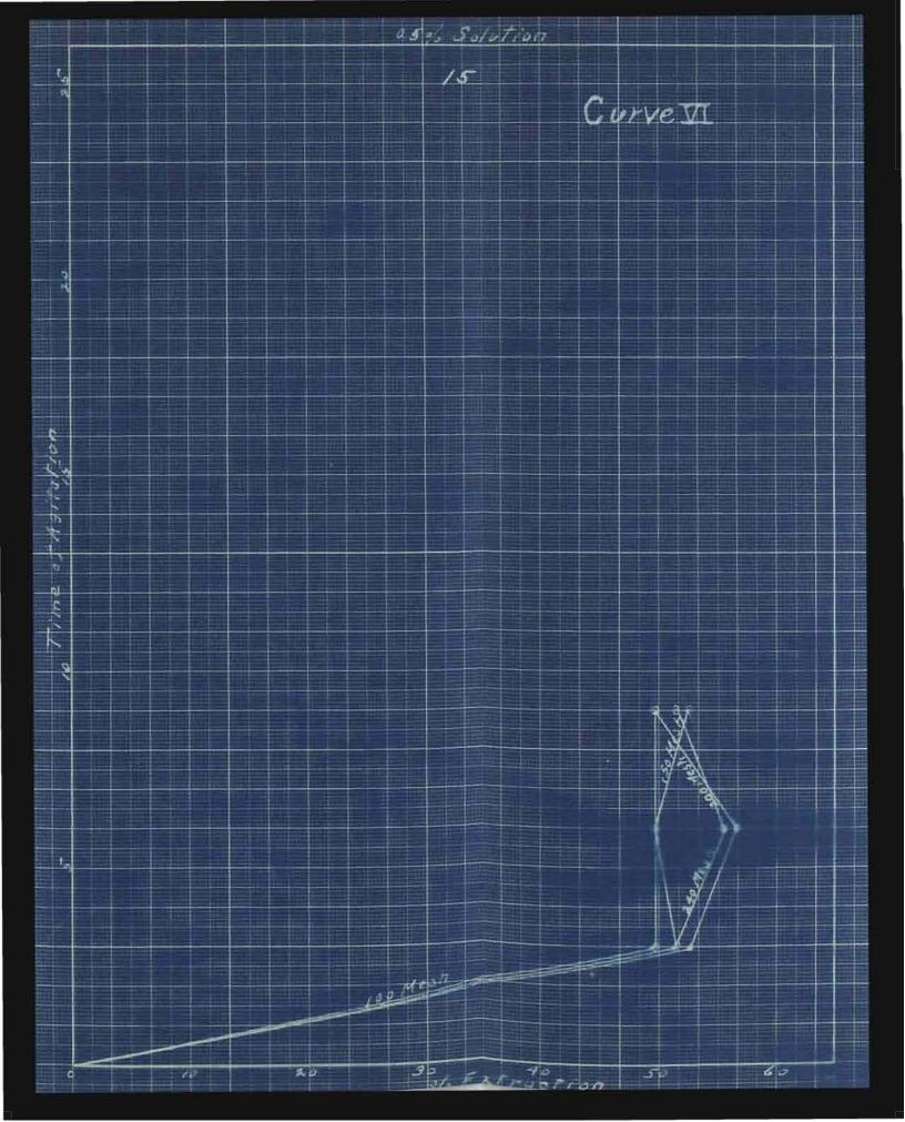
The KCN consumption (6.5#s per ton) is high. A test was made on some of the solution to determine what substances were acting as cyanicides. The test showed that copper was the large consumer. A small amount of antimony was also found to be present.
