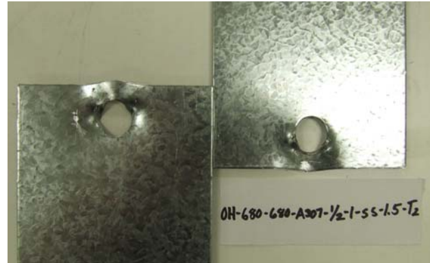
Fig 9-10 Sheet Shear Failure of a 68 mil Single Shear Connection with One A307 Bolt
