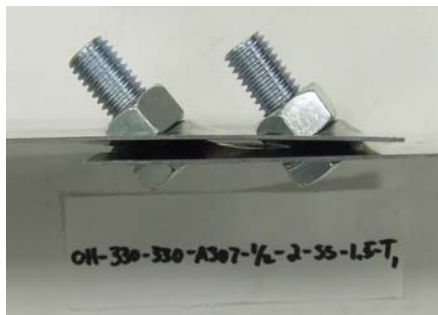
Fig 8-11 Failure Mode of Test OH-330-330-A307-1/2-2-SS-1.5-T1
