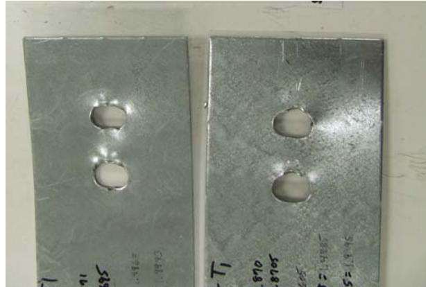
Fig 8-22 Failure Mode of Test SS-118-118-A307-9/16x7/8-2-SS-4-T1
