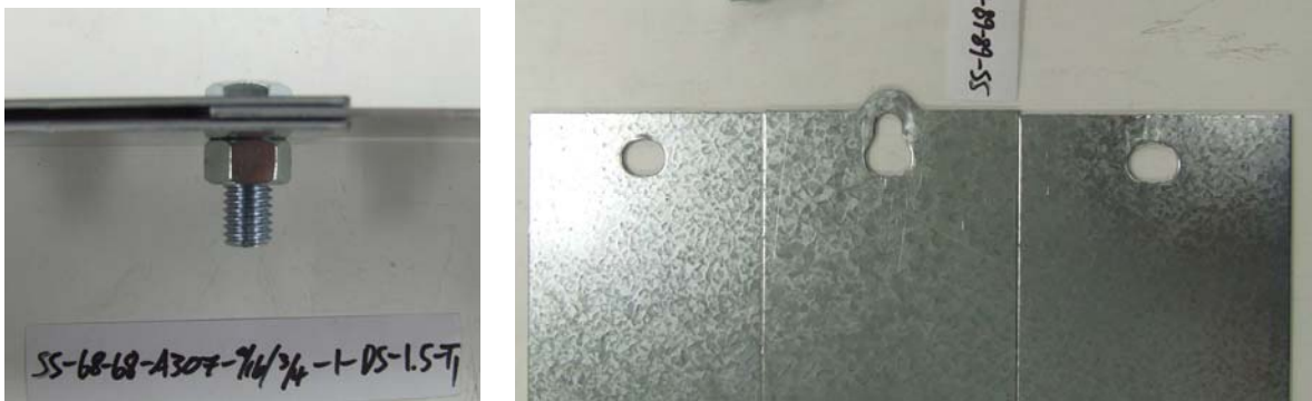
Fig 8-37 Failure Mode of Test SS-68-68-A307-9/16x3/4-1-DS-1.5-T1
