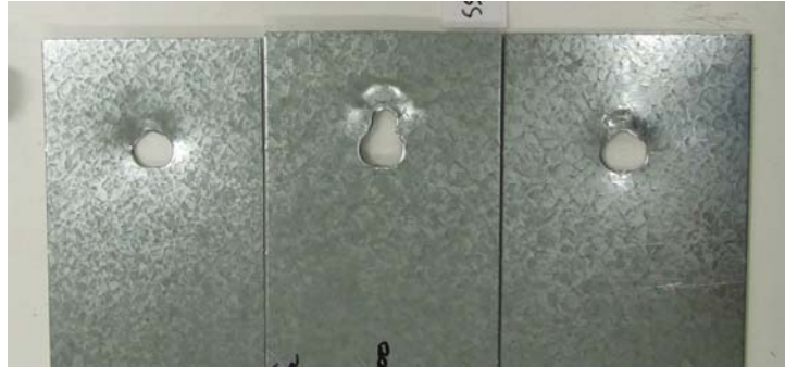
Fig 8-26 Failure Mode of Test SS-68-68-A307-9/16x3/4-1-DS-4-T2
