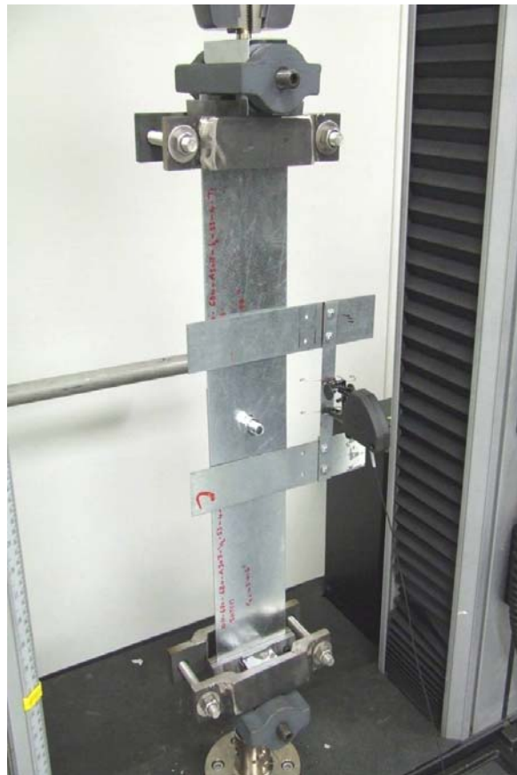
Fig 6-1 Setup for Tensile Tests on Bolted Connections
