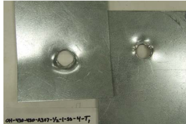
Fig 9-6 43 mil High Ductile Steel Bearing Failure
