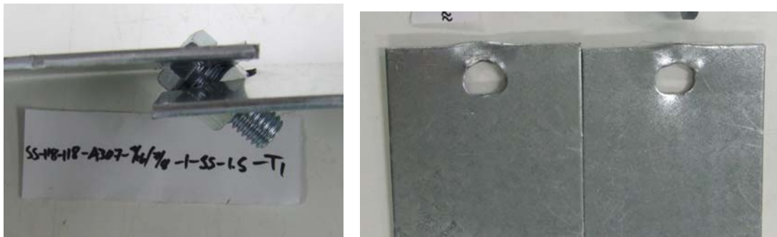
Fig 8-32 Failure Mode of Test SS-118-118-A307-9/16x7/8-1-SS-1.5-T1
