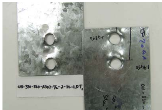
Fig 8-11 Failure Mode of Test OH-330-330-A307-1/2-2-SS-1.5-T1
