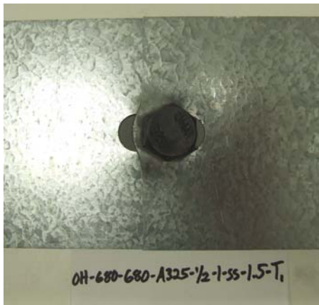
Fig 9-11 Sheet Shear Failure of a 68 mil Single Shear Connection with One A325 Bolt
