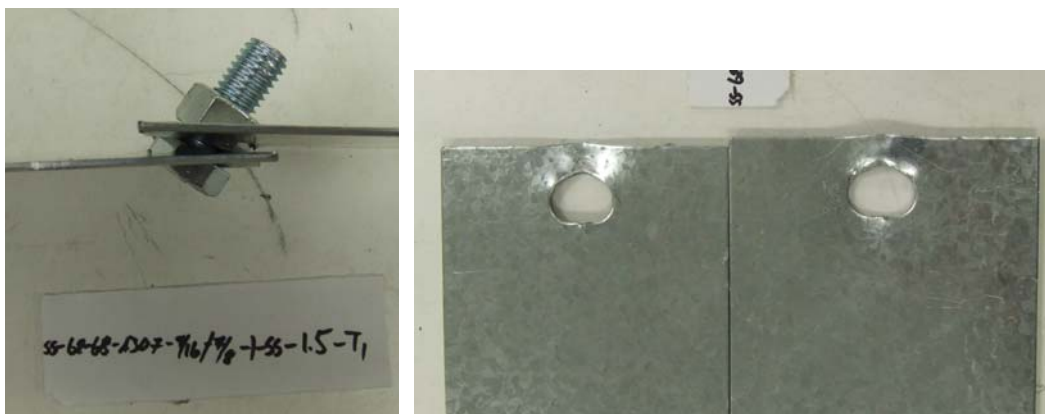
Fig 8-33 Failure Mode of Test SS-68-68-A307-9/16x7/8-1-SS-1.5-T1
