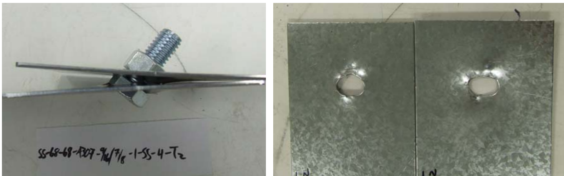
Fig 8-18 Failure Mode of Test SS-68-68-A307-9/16x7/8-1-SS-4-T2
