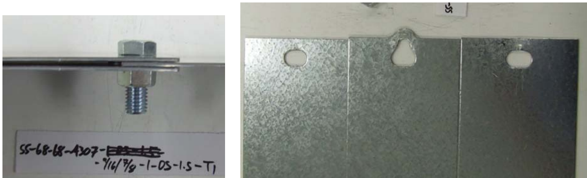
Fig 8-38 Failure Mode of Test SS-68-68-A307-9/16x7/8-1-DS-1.5-T1
