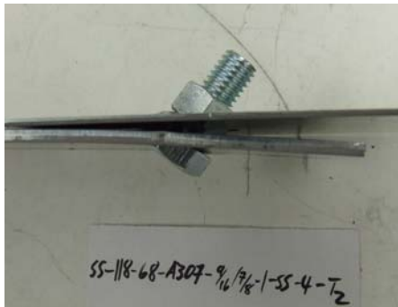
Fig 8-23 Failure Mode of Test SS-118-68-A307-9/16x7/8-1-SS-4-T2
