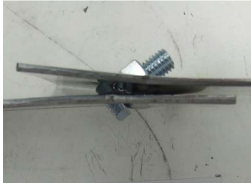
Fig 8-19 Failure Mode of Test SS-118-118-A307-9/16x3/4-1-SS-4-T2
