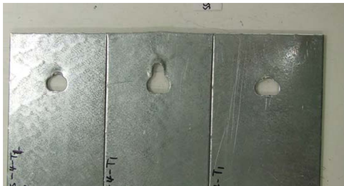
Fig 8-29 Failure Mode of Test SS-118-118-A307-9/16x7/8-1-DS-4-T1
