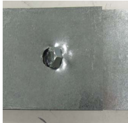
Fig 8-19 Failure Mode of Test SS-118-118-A307-9/16x3/4-1-SS-4-T2
