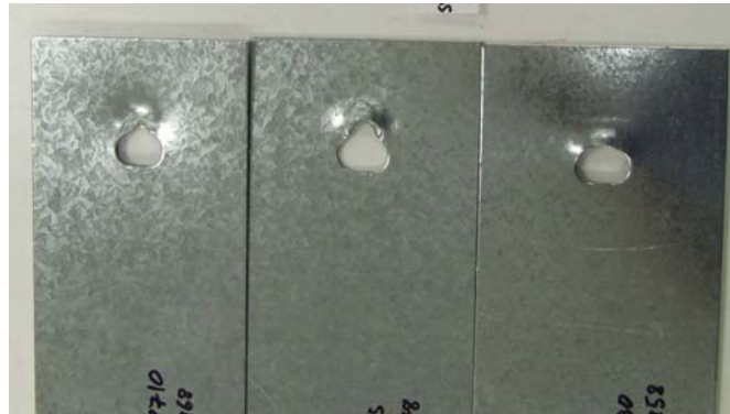
Fig 8-27 Failure Mode of Test SS-68-68-A307-9/16x7/8-1-DS-4-T1
