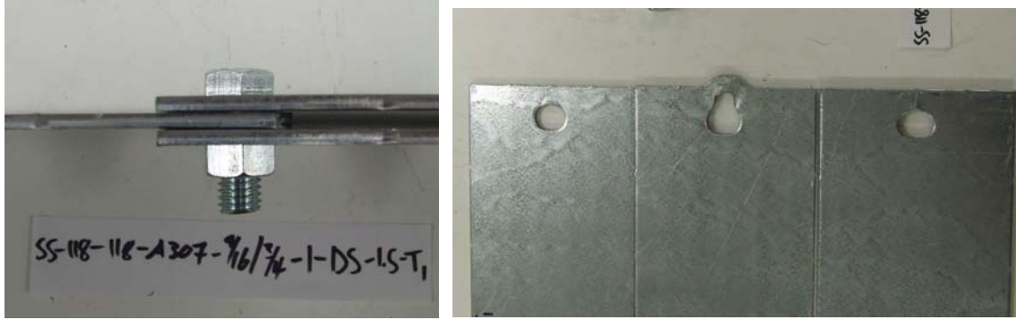
Fig 8-35 Failure Mode of Test SS-118-118-A307-9/16x3/4-1-DS-1.5-T1
