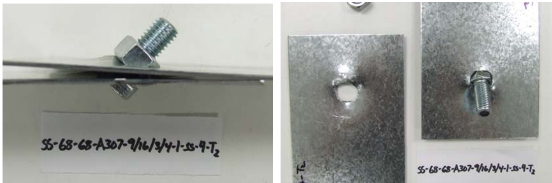
Fig 8-17 Failure Mode of Test SS-68-68-A307-9/16x3/4-1-SS-4-T2
