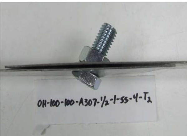
Fig 9-7 39 mil Low Ductile steel Bearing Failure
