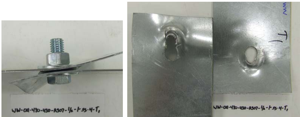
Fig 8-14 Failure Mode of Test WW-OH-43O-43O-A307-1/2-1-SS-4-T1
