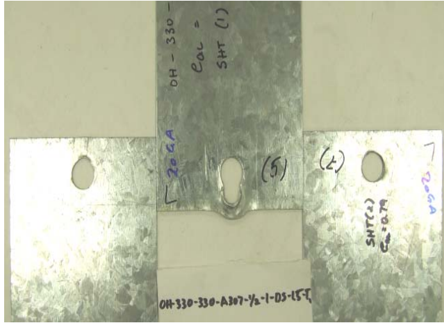
Fig 8-9 Sheet Shear Failure of Double Shear Connection OH-330-330-A307-1/2-1-DS-1.5-T1
