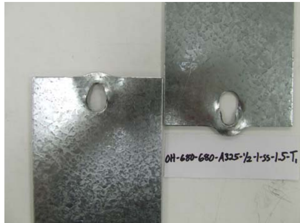
Fig 9-11 Sheet Shear Failure of a 68 mil Single Shear Connection with One A325 Bolt
