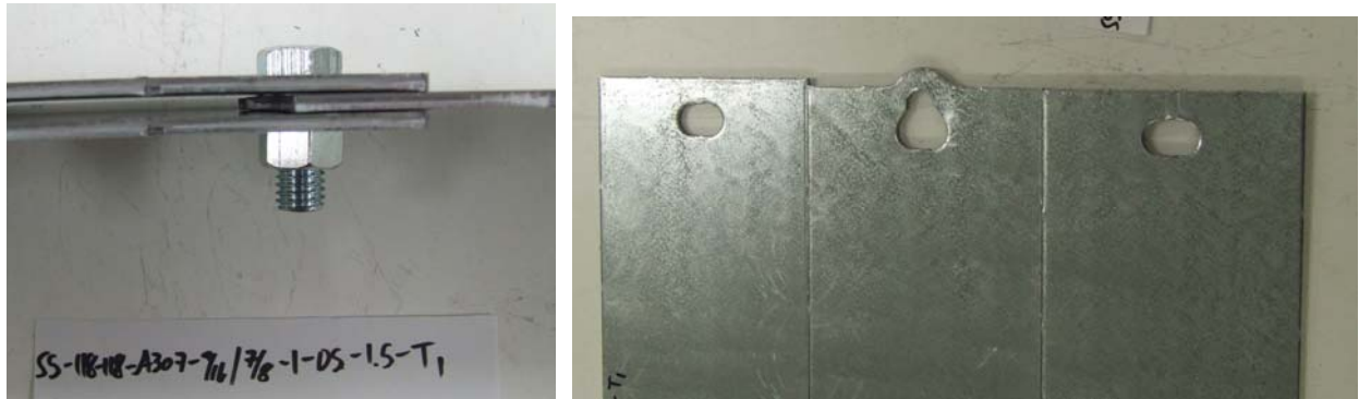
Fig 8-36 Failure Mode of Test SS-118-118-A307-9/16x7/8-1-DS-1.5-T1
