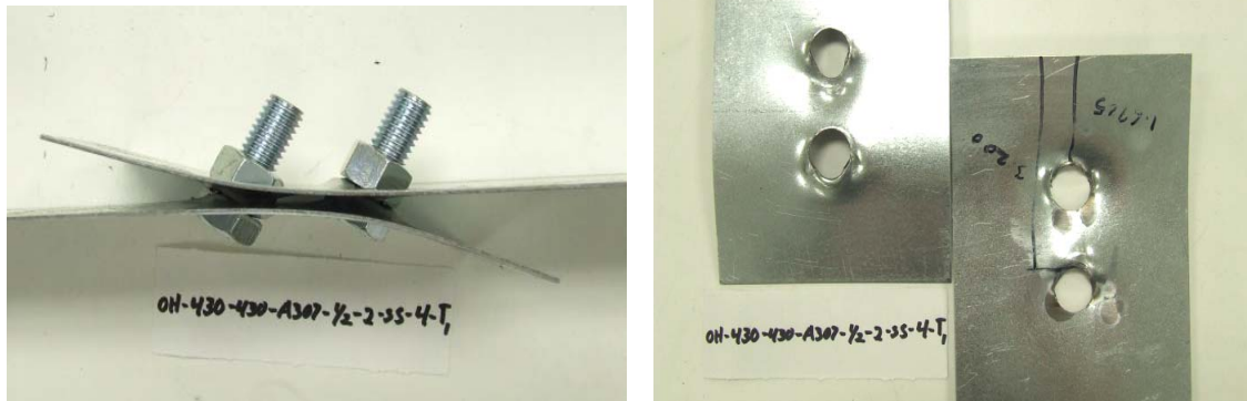
Fig 8-5 Sheet Bearing Failure of Single Shear Connection OH-430-430-A307-1/2-2-SS-4-T1
