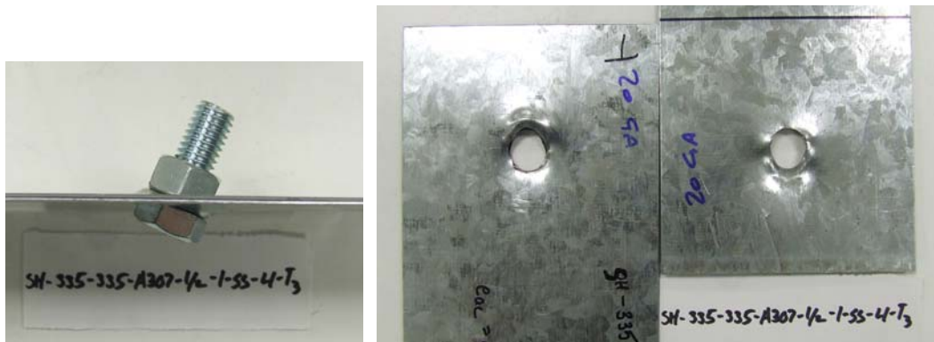
Fig 8-15 Failure Mode of Test SH-33S-33S-A307-1/2-1-SS-4-T3
