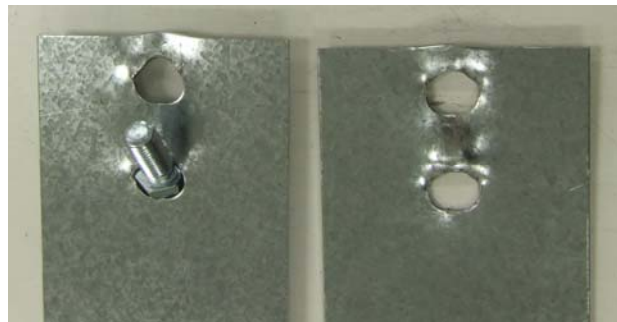
Fig 8-39 Failure Mode of Test SS-68-68-A307-9/16x3/4-2-SS-1.5-T3
