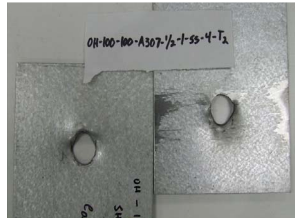
Fig 9-7 39 mil Low Ductile steel Bearing Failure
