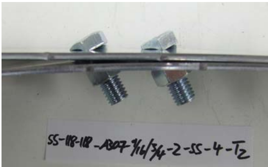
Fig 8-21 Failure Mode of Test SS-118-118-A307-9/16x3/4-2-SS-4-T2
