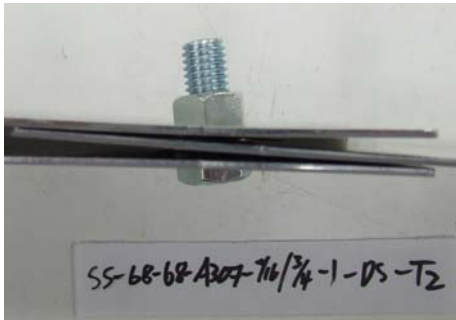
Fig 8-26 Failure Mode of Test SS-68-68-A307-9/16x3/4-1-DS-4-T2
