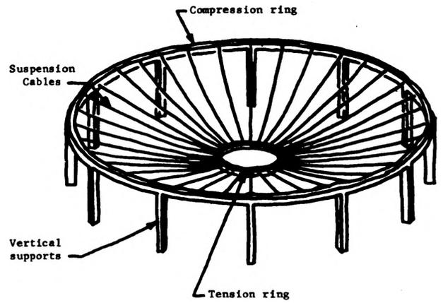
Fig. 2. Cable-Suspended Roof
