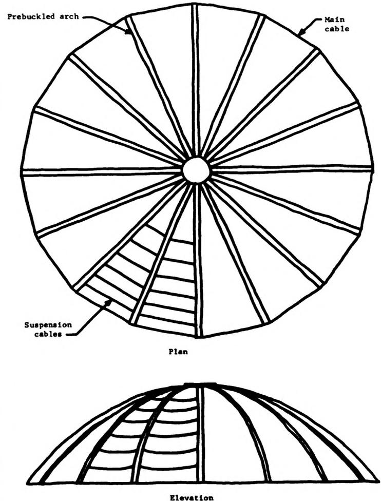
Fig. 3. Semi-rigid Prebuckled Dome
