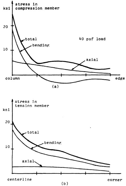
FIG. 3 CALCULATED STRESSES IN THE EDGE MEMBERS OF AN UMBRELLA STRUCTURE
