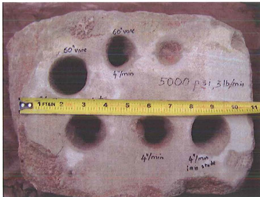
Figure 6.14. Testing influence of vane angle, AFR and pressure
