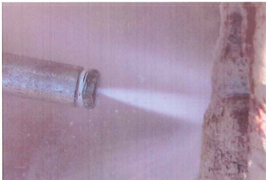
Figure 6.15. Effect of water, abrasive and rock exiting the hole
