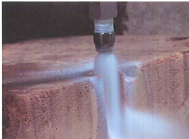
Figure 7.5. Supercritical \text{CO}_2 jet carrying abrasive cutting into Roubideaux sandstone
