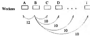
**Figure B.2:** Bound received by worker A is greater than all the others.
