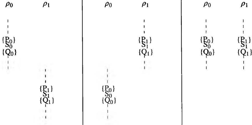
Figure 3.2. Some possible process execution sequences before communication takes place.
