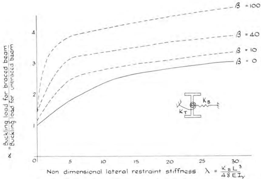
FIG. 5 EFFECT OF A COMBINED CONTINUOUS RESTRAINT ON A BEAM FOR WHICH  $R^2 = 100$
