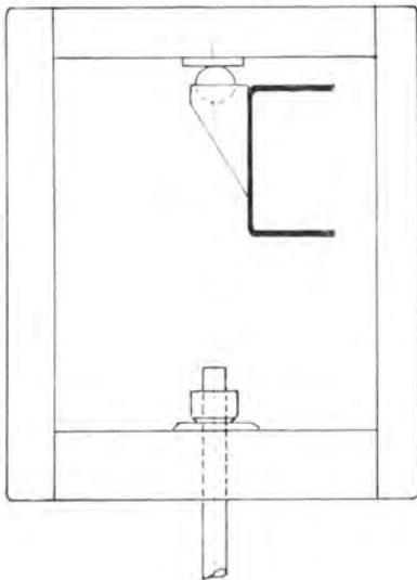
FIG. 7 LOADING YOKE
