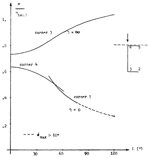
FIG. 9a Comparison of the moment  $M$  when stress reaches  $1.15 \sigma_y$
