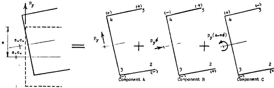
FIG. 11a Components of the vertical uplift load for unbraced channel
