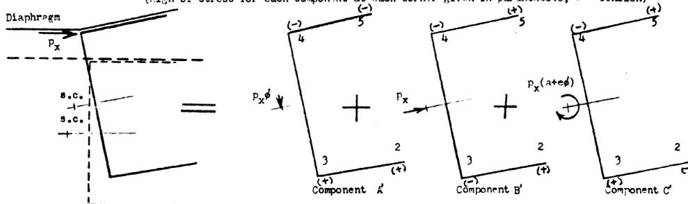
FIG. 11b Components of bracing force
