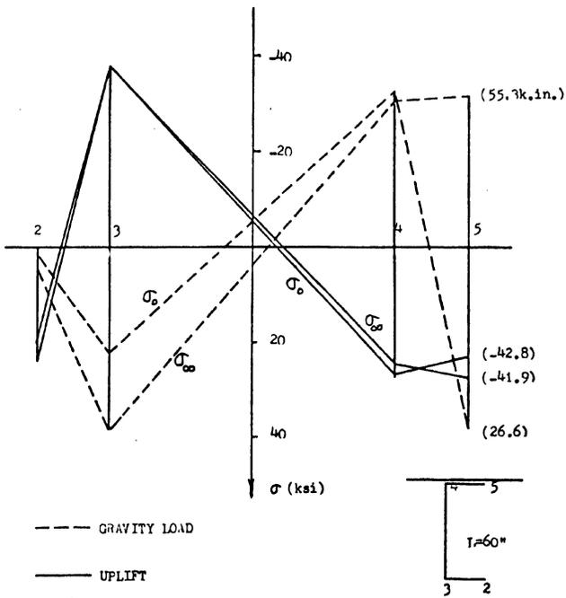
FIG. 12 Stress distribution at failure
