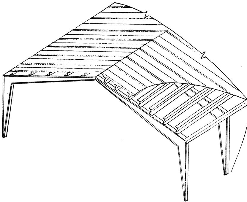
FIG. 1 Roof assembly with diaphragm braced Z-section purlins
