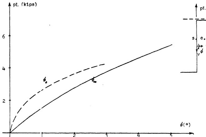
FIG. 8a Midspan rotation  $\phi$  versus  $pL$  upto theoretical failure
