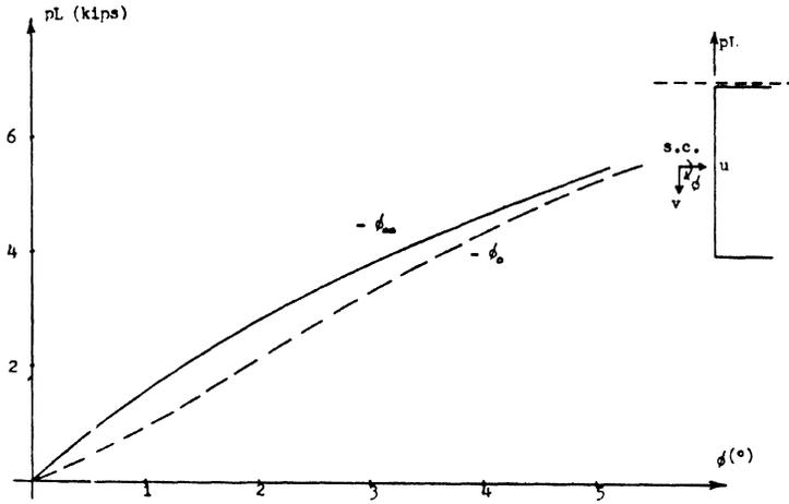
FIG. 7a Mid-span rotation  $\phi$  versus  $pL$  upto theoretical failure
