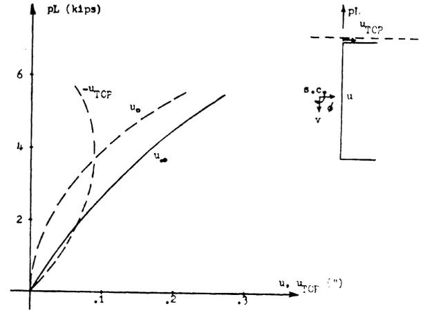
FIG. 7b Lateral deflection  $u$  versus  $pL$  upto theoretical failure
