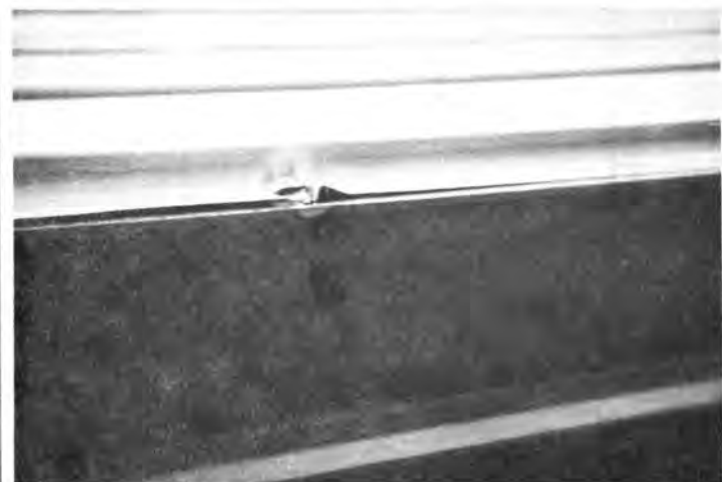
Fig. 10 Sheet Tearing and Displacement
