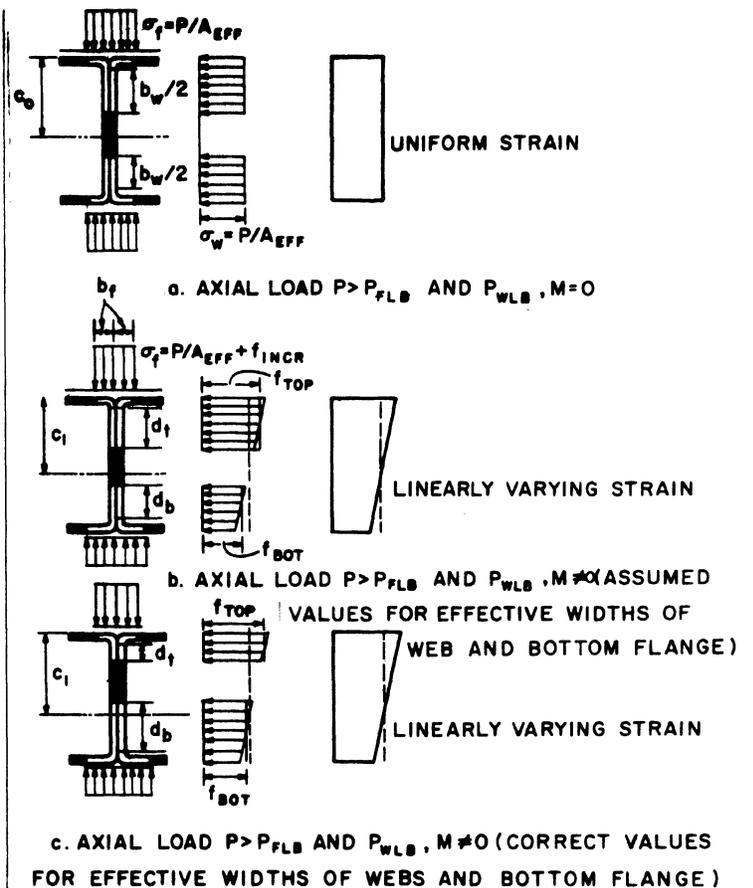
Fig. 2 Stress and Strain Distribution Over Cross Section
