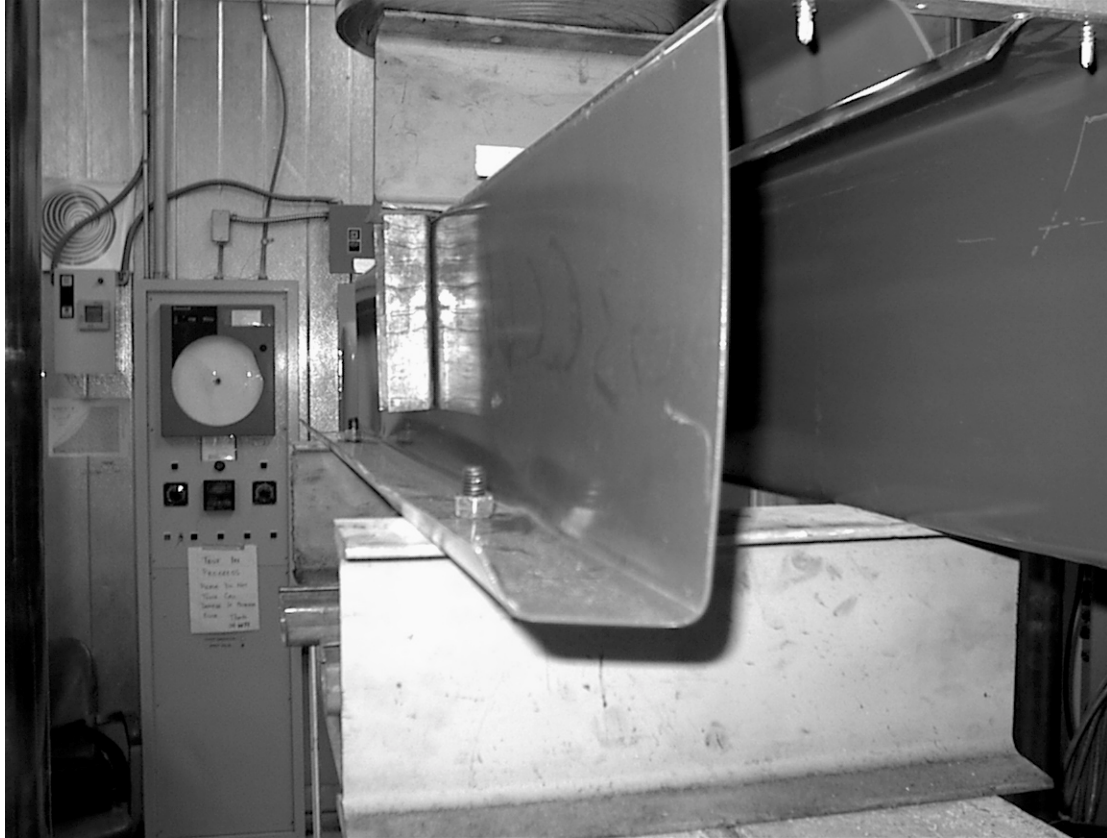
Figure 3.4. Local Yielding of Test Specimen
