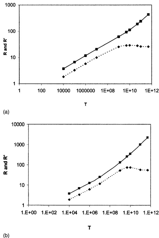
FIG. 5. (a) The contact line measured with two different dimensionless resolutions has been shown for  $h_0=100$  nm. The lower line which attains equilibrium is for a dimensionless resolution of  $\pm 0.5$  ( $R'$  dashed line), while the upper line which continues to rise is for a resolution of  $\pm 0.01$  ( $R$  bold line). (b) The same as in Fig. 5(a) for  $h_0=50$  nm.
