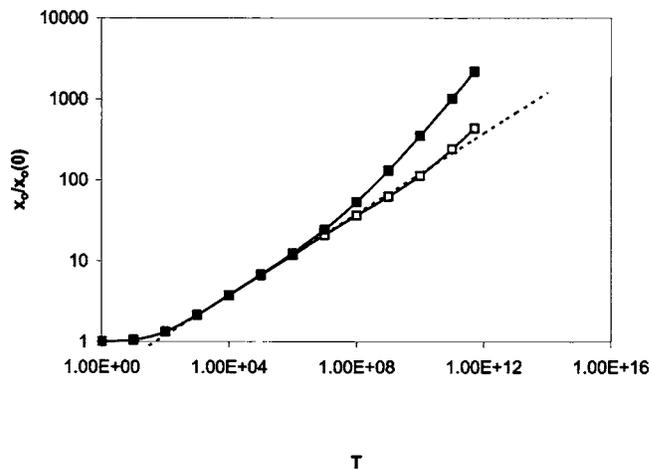
FIG. 2. The results for liquid-containing polymers have been shown for the two cases of  $h_0=100$  nm (white squares) and  $h_0=50$  nm (solid black squares). The dashed line represents the asymptotic  $\frac{1}{4}$  slope, which is an indication of surface-tension-driven flow. At larger times the slope increases to a power of  $\frac{1}{2}$ , which is disjoining-pressure-driven flow determined by Hamaker forces only.
