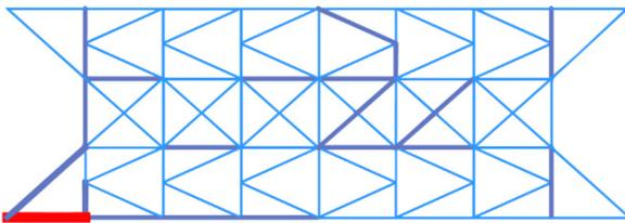
**Figure 4: MetaGA tours for 4 robots on a K truss.**
