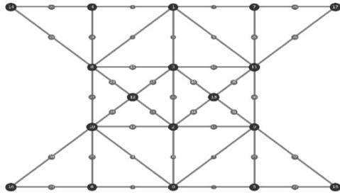
**Figure 3: Mapping a Pratt truss to a corresponding graph.**
