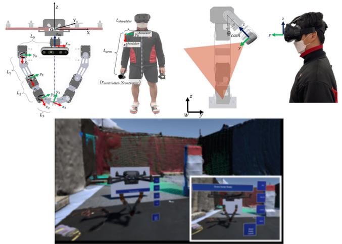
**Figure 2: Human arm/head and aerial manipulator kinematic matching (Top), virtual test-site, aerial manipulator rendered in VR headset (Bottom).**
