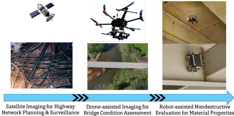
Figure 5: A multiscale sensing system for condition assessment of a bridge network.
