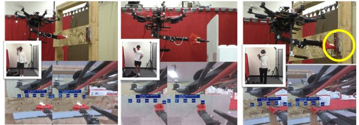
**Figure 5: Flight trials: peg-in-hole (left), drilling (center), key manipulation (Right)**
