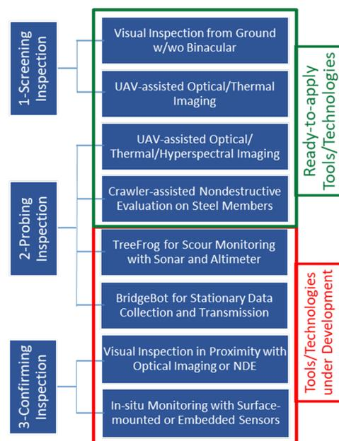
Figure 3: A robot-assisted inspection protocol.
