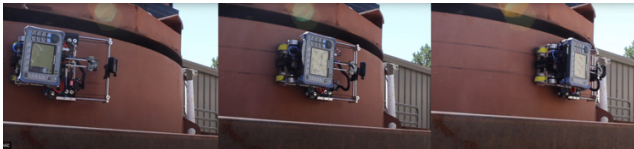
Figure 4. Robot testing on a curved steel surface.
