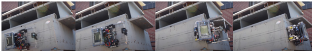
Figure 5. Testing the robot on a flat steel structure and pass the angle 90°.
