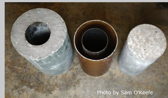
From the left: ElGawady’s concrete column, the steel tube and polymer without concrete, and the current standard.
