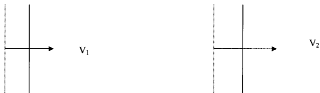
FIG. 2. Cathode on the left and the anode to the right, moving at unequal rates.
