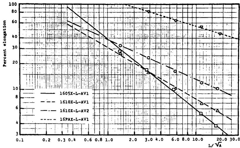
Fig. 3. Elongation -  $L/\sqrt{A}$  curves for 16 gage X steel.
