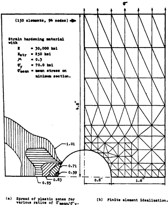
Fig. 7. Perforated tension strip ( $d/s = 0.33$ ), plane stress.
