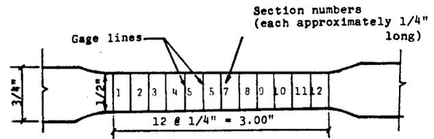
Fig. 2a. Sketch of a standard tension coupon.
