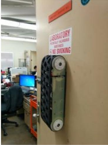
**Rise-Rover:** a wall-climbing robot to carry heavy NDT instruments (>50lb) for visual and contact-based inspection.
