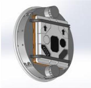
**GPR-Rovers:** custom designed wall-climbing robots to carry GSSI's ground penetrating radar (GPR) for detecting subsurface defects, locating rebar and pipes.
