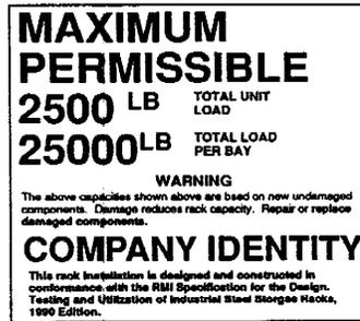
Figure 1.4.2a Example of Load Capacity and Compliance Plaque.
