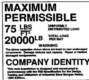
Figure 1.4.2b Example of Load Capacity and Compliance Plaque.
