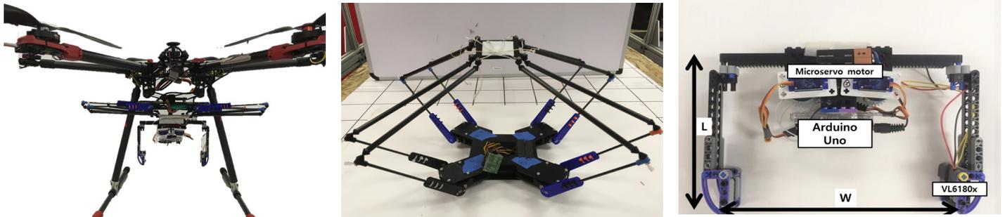
**Fig. 1. Parallel-based arm (middle) and gripper (right) in stowed position on rotorcraft (left)**
