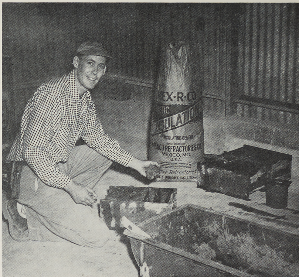
John Young making test bars in the control laboratory of the Mexico Refractories Company at Mexico, Missouri.
