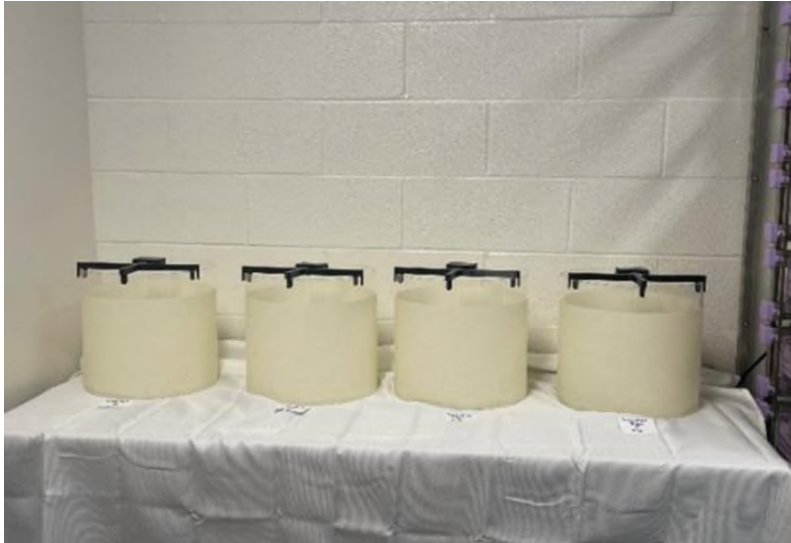
Figure 3. Specially built chambers for video recording of mice. These specially built recording chambers hold a Go Pro video camera in the mount on the top and are covered on the side to prevent any behavior alteration of the mouse due to outside activity.
