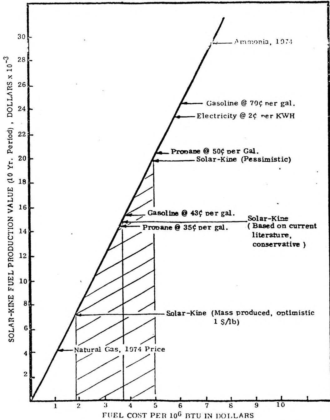
Figure 4. Cost Analysis of the Solar-Kine Based on the Replaced Fuel Value
