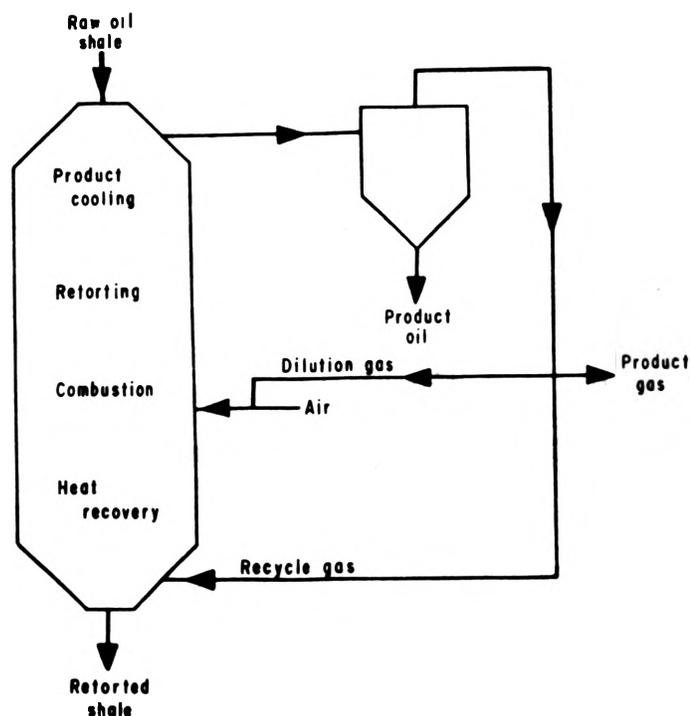
Fig. 4. Gas combustion retort.
