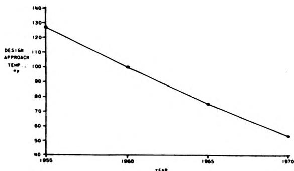
Fig. 3. Cat. reformer design approach temperatures
