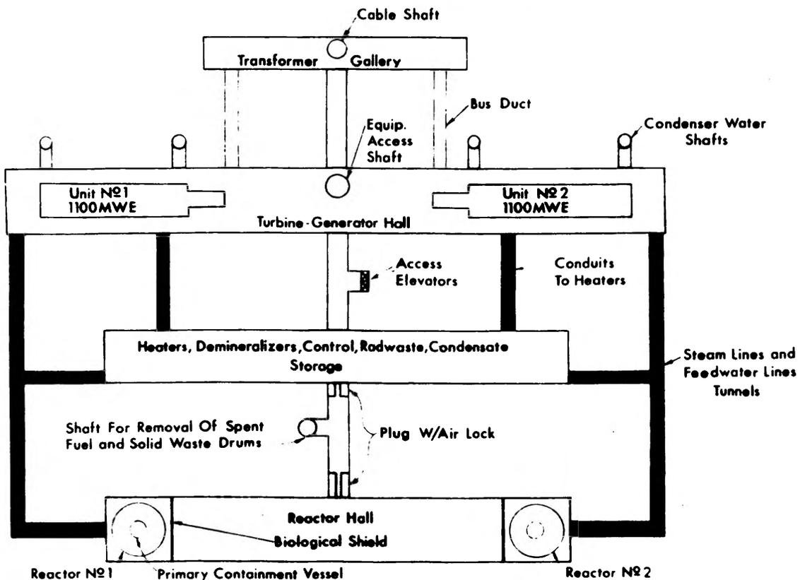
FIG. 6 UNDERGROUND NUCLEAR PLANT
