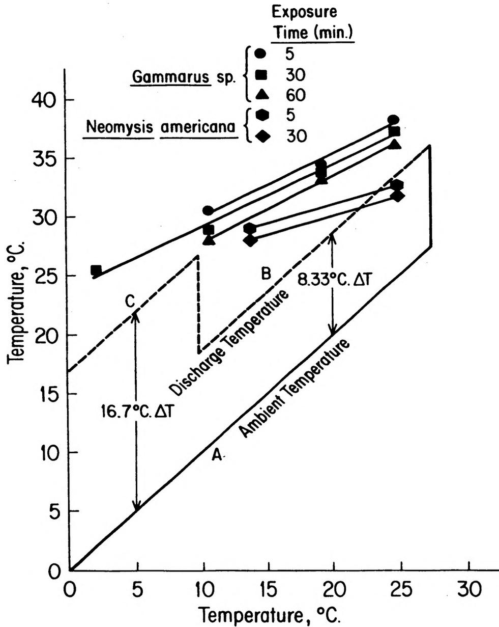
Figure 5. 95% tolerance limits for *Gammarus* sp. and *Neomysis americana*. Projected power plant  $\Delta T$ 's during full flow (line B) and reduced flow (line C) operations are superimposed over the ambient temperature range (line A).
