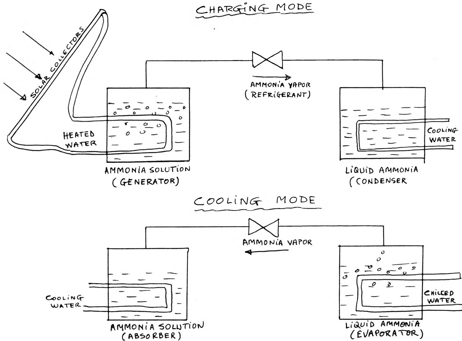
Figure 4. Schematic diagram for a  $\text{NH}_3\text{-H}_2\text{O}$  absorption air-conditioner
