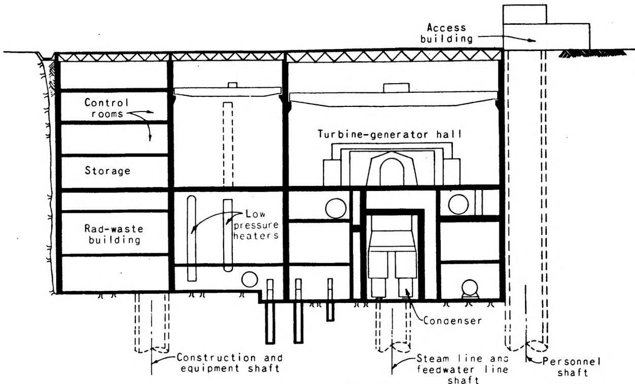
FIG. 5 TURBINE GENERATOR STRUCTURE
