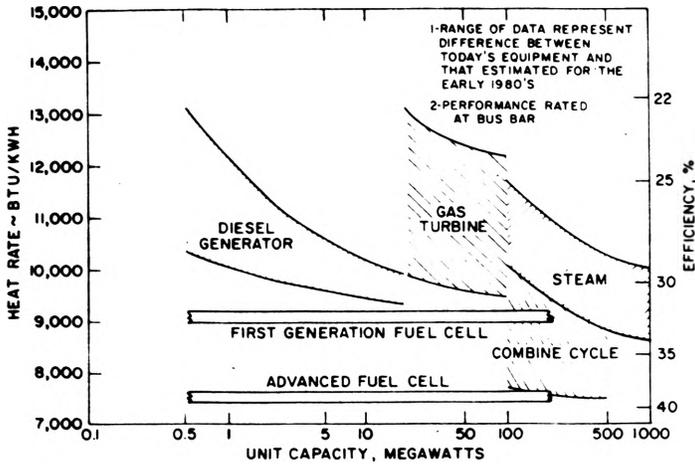
Fig. 5. Energy Systems Comparison (Performance vs. Unit Size)
