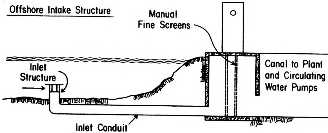
**Figure 1. Schematic Diagrams of Typical Intake Structures
