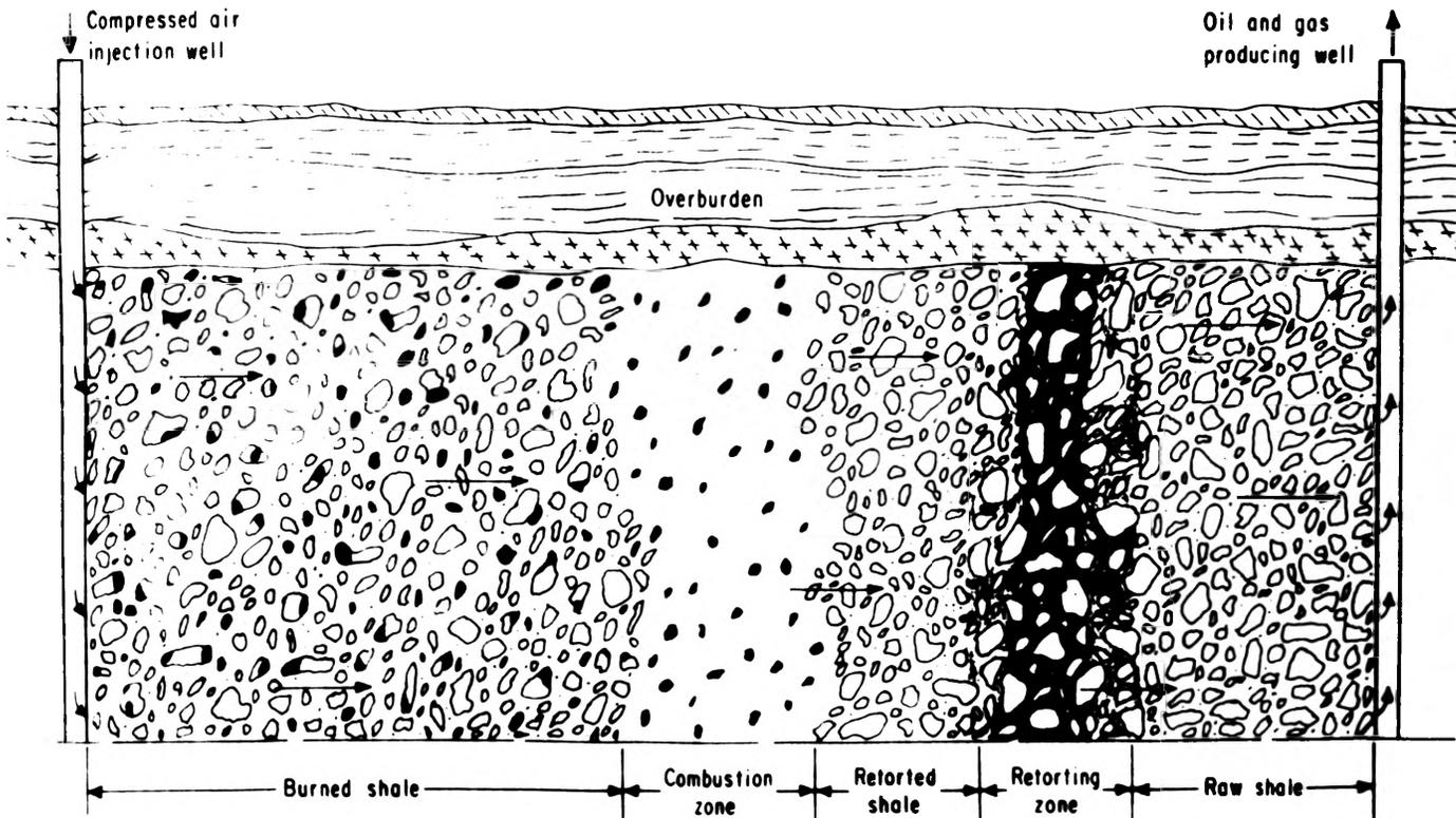
Fig. 5. Schematic diagram of an in situ oil shale retorting process
