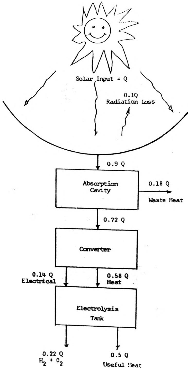
FIG. 3. Solar Hydrogen Production System.
