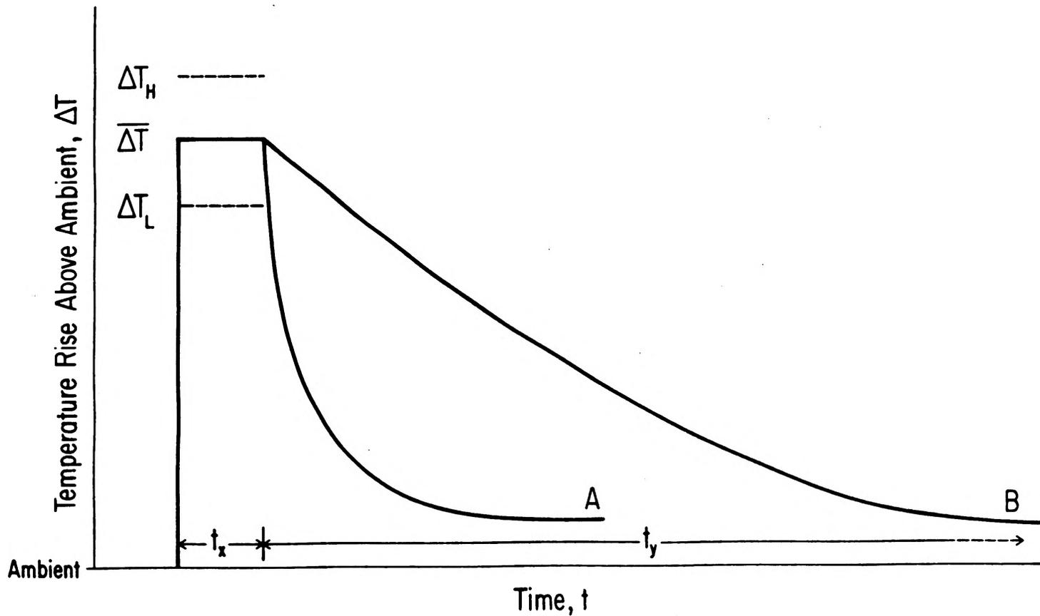
Figure 2. Generalized temperature exposure diagram for organisms entrained in a once-through, steam electric power plant cooling system.  $\Delta T_L$  and  $\Delta T_H$  represent the range and  $\Delta T$  the average temperature increase experienced in the condenser. Inplant and post-discharge exposure times are represented by  $t_x$  and  $t_y$ , respectively. Curves A and B represent high and low rates of mixing, respectively.
